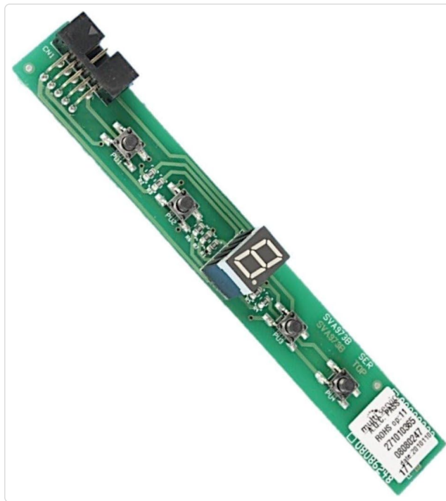
Image: Best Airlux Control Module 08080247. This image displays the green circuit board with several black push buttons (labeled PU1, PU2, PU3, PU4), a 7-segment digital display, and a multi-pin connector (CN1) at one end. Various electronic components are visible on the board.
