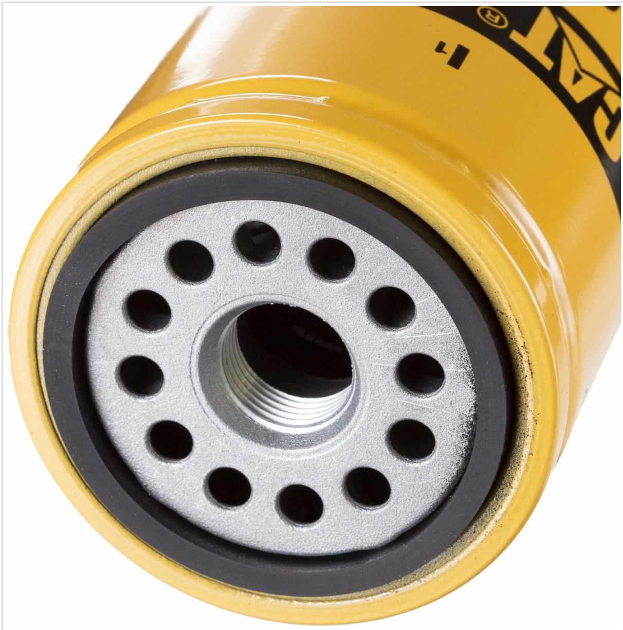
Figure 2: Close-up of the filter's threaded end, showing the gasket and thread size (7/8-14-2B).
