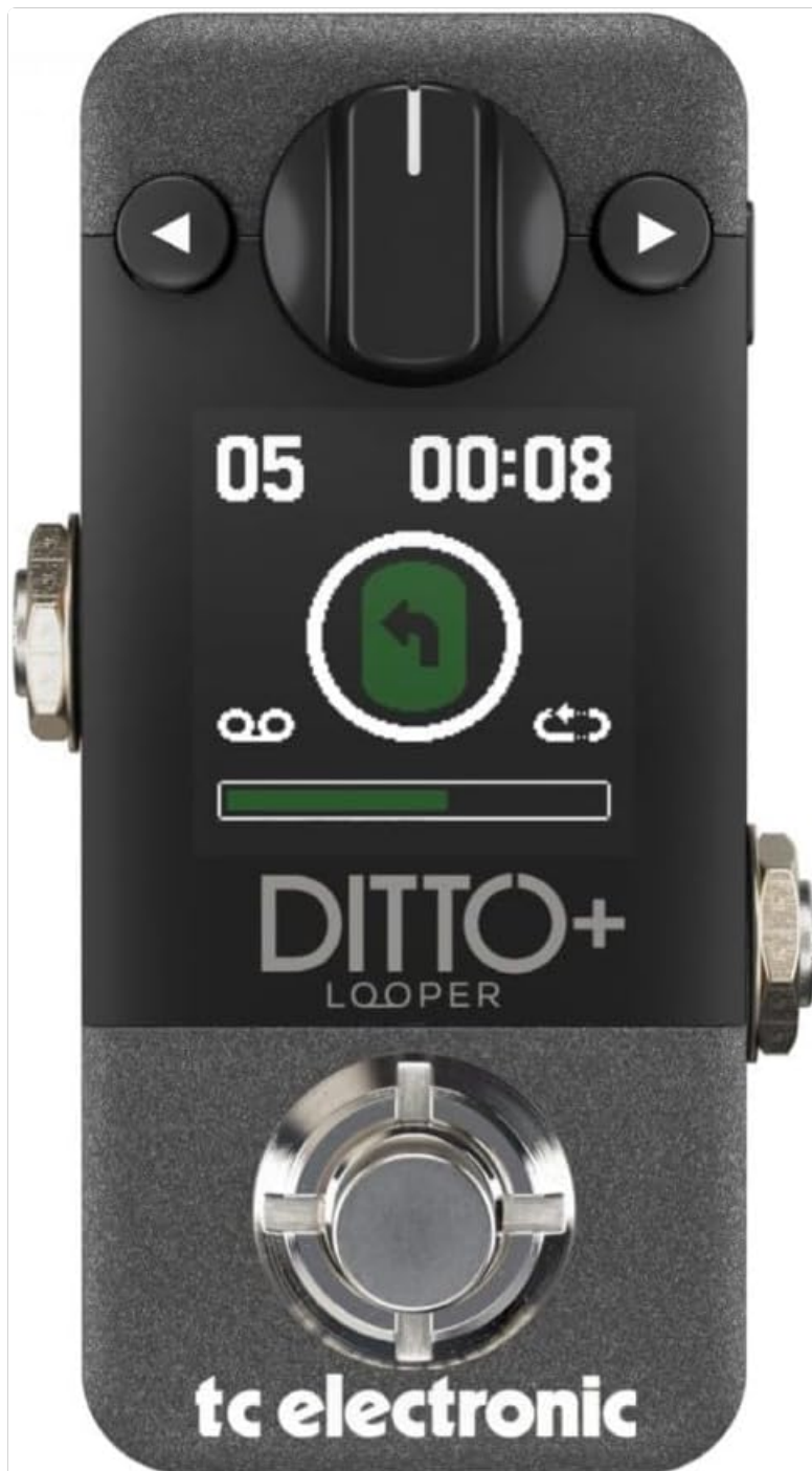
Image 3: Front view of the Ditto+ pedal, displaying the main screen, the large central knob, the two arrow buttons, and the footswitch. This image illustrates the primary user interface.
