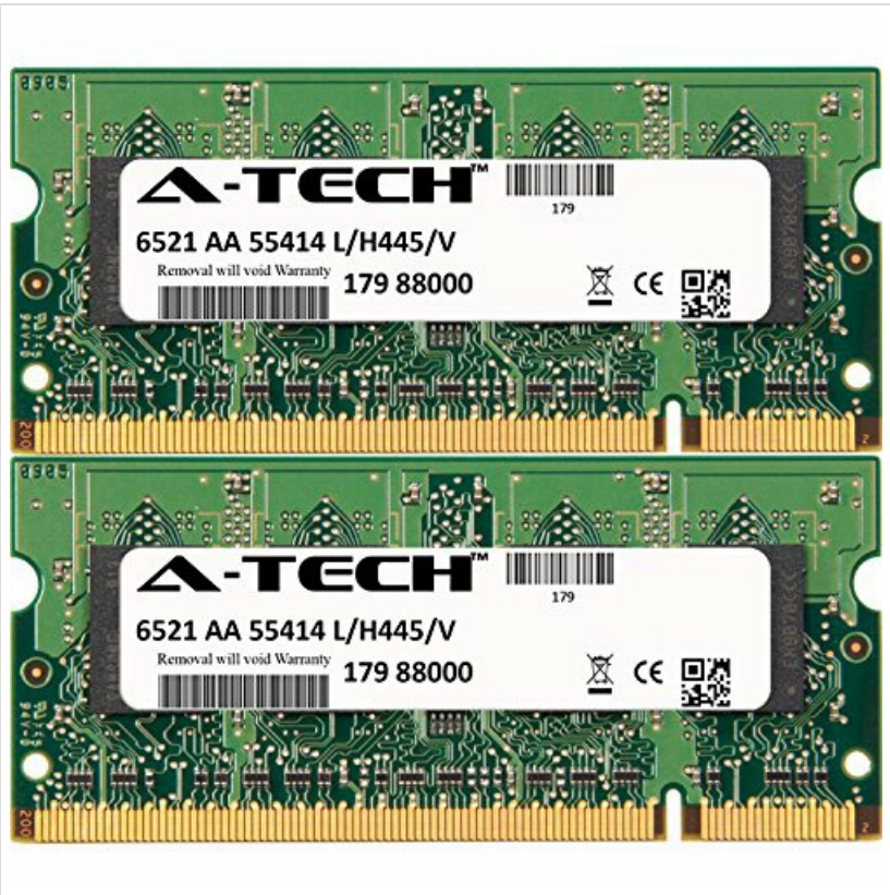
Image: A single A-Tech 2GB DDR2 SO-DIMM RAM module, showing the green PCB and black memory chips.
