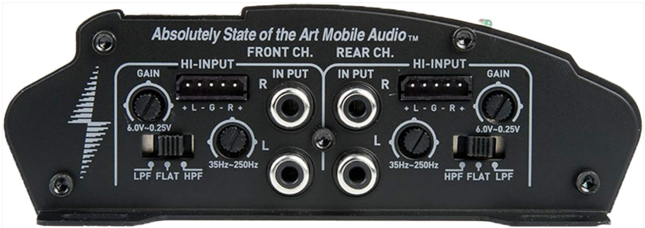
Figure 3: Input panel of the Precision Power i1000.4 amplifier, displaying gain controls, RCA inputs, and crossover switches for front and rear channels.
