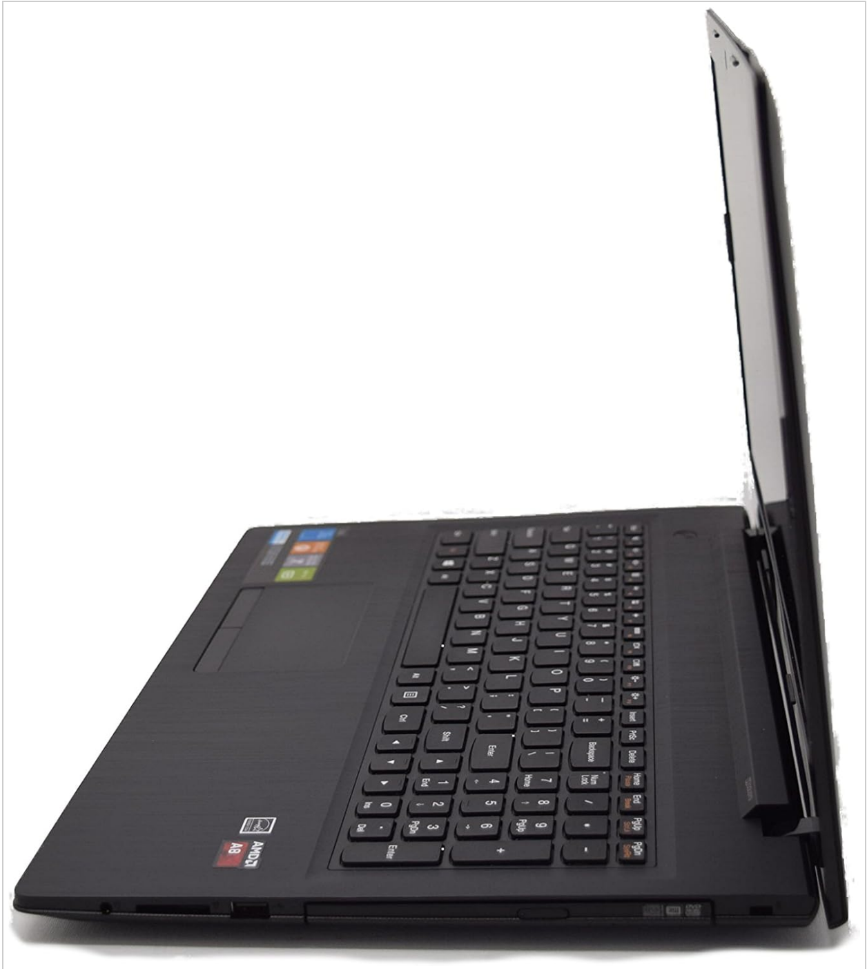
A side view of the Lenovo G50 80E30181US laptop, displaying the DVD-SuperMulti drive and two USB 2.0 ports on the right side.
