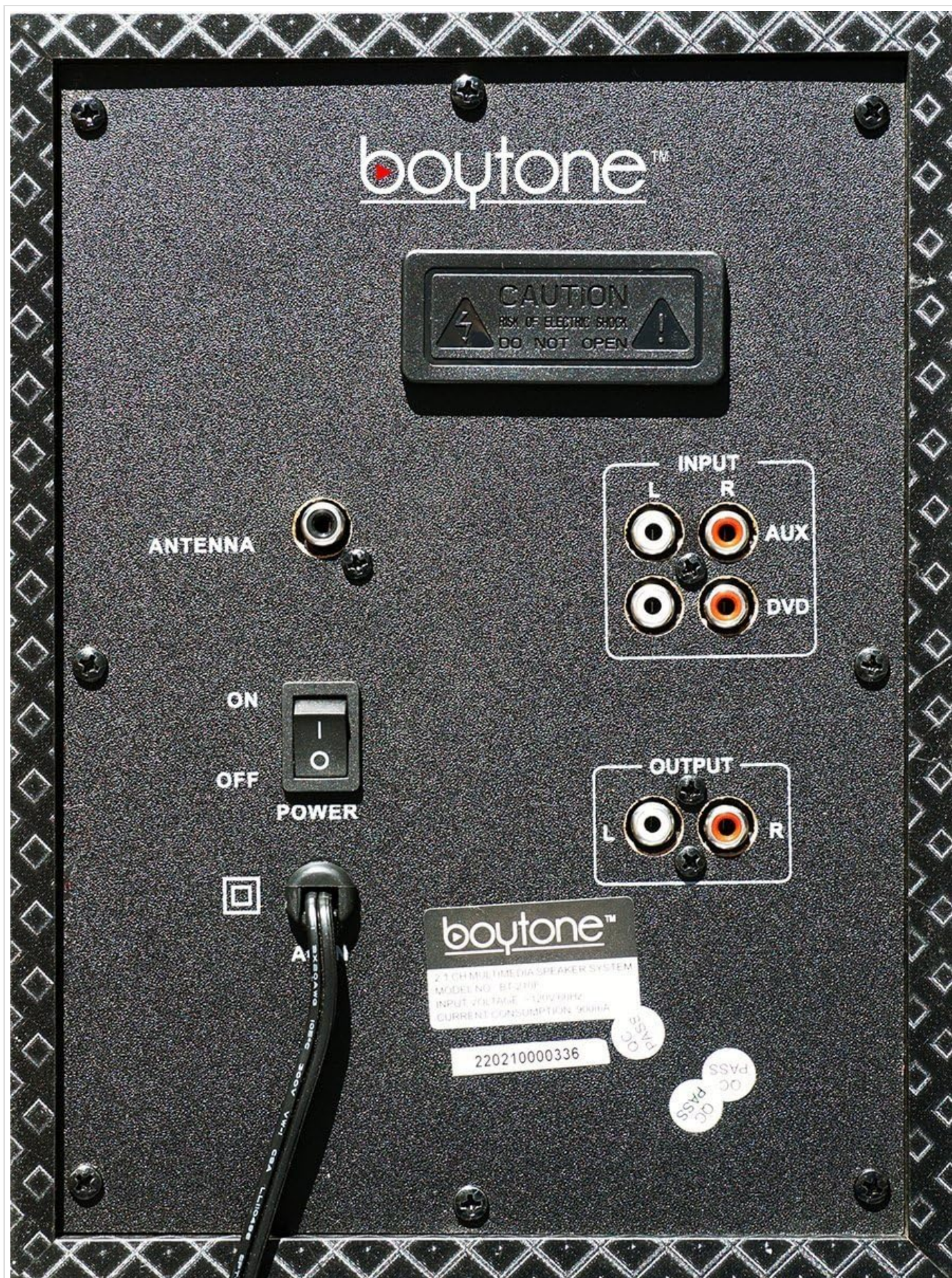
Figure 3: Rear panel of the subwoofer unit, showing speaker outputs, AUX/DVD inputs, FM antenna port, and power switch.
