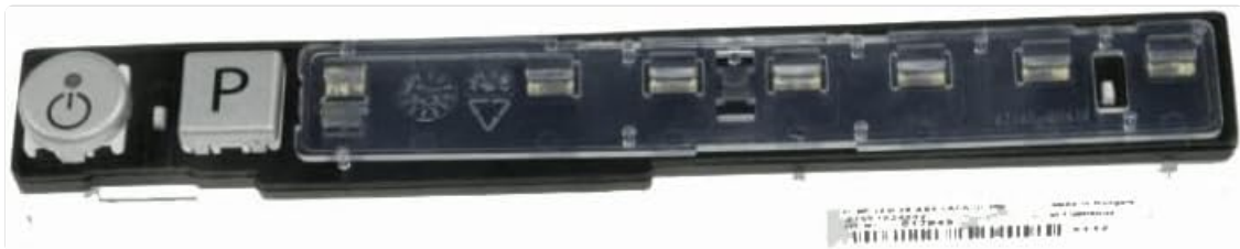
Figure 1: Hotpoint LED Control Card C00297080. This image shows the rectangular control card with a grey power button on the left, a grey 'P' button next to it, and a clear plastic cover revealing LED indicators and internal components along the right side.
