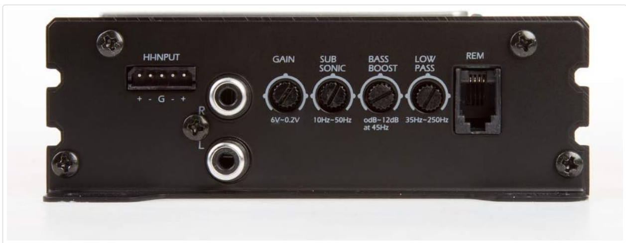
Figure 2: Input and Control Panel. This view shows the amplifier's input and adjustment section. From left to right, you can see the HI-INPUT terminal, RCA input jacks (L/R), GAIN control (6V-0.2V), SUB SONIC filter (10Hz-50Hz), BASS BOOST control (0dB-12dB at 45Hz), LOW PASS filter (35Hz-250Hz), and the REM (Remote) port for the wired bass control.
