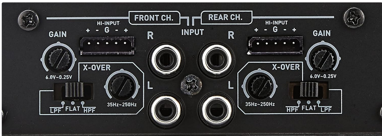
Image 5.1: Close-up of the amplifier's control panel, showing gain knobs, crossover switches (LPF, FLAT, HPF), and input connections for both front and rear channels.
