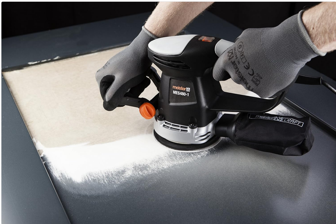
Figure 5: Proper technique for sanding a wooden surface, showing two-hand grip.
