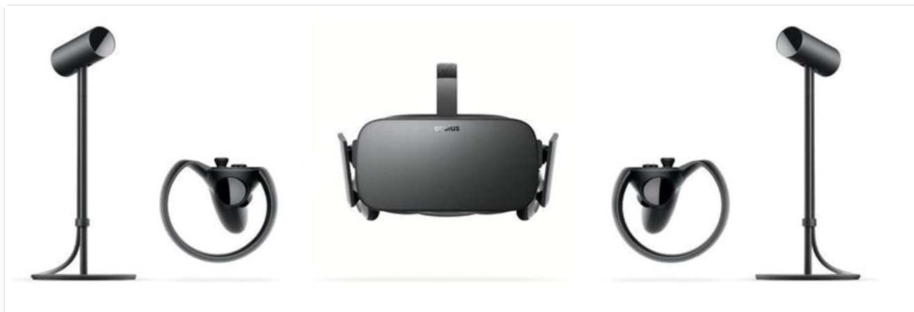
Figure 1: The Oculus Rift headset and its primary components.
