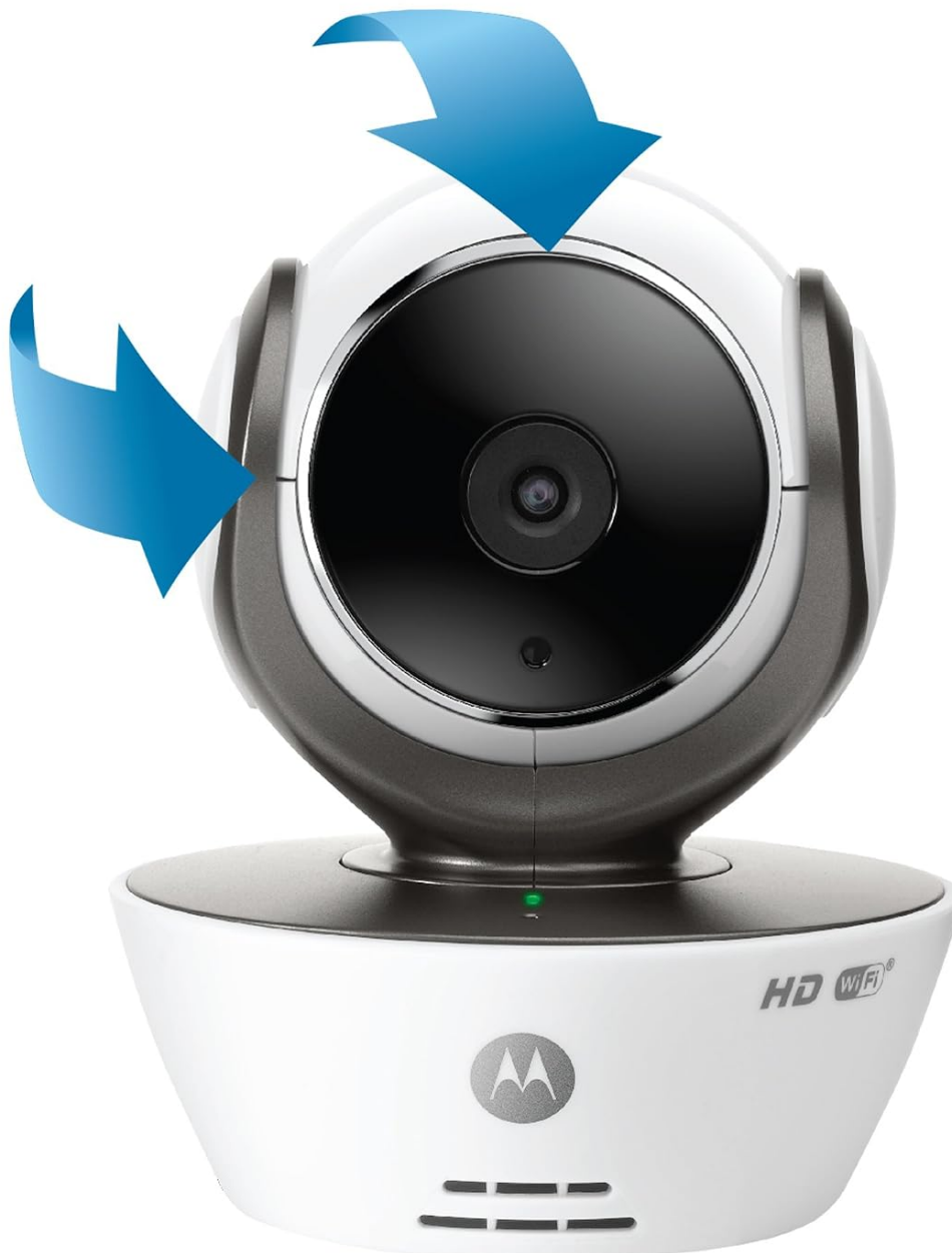
Image 3.2: The Motorola MBP853CONNECT Baby Unit (camera), illustrating its remote pan and tilt functionality with blue arrows.
