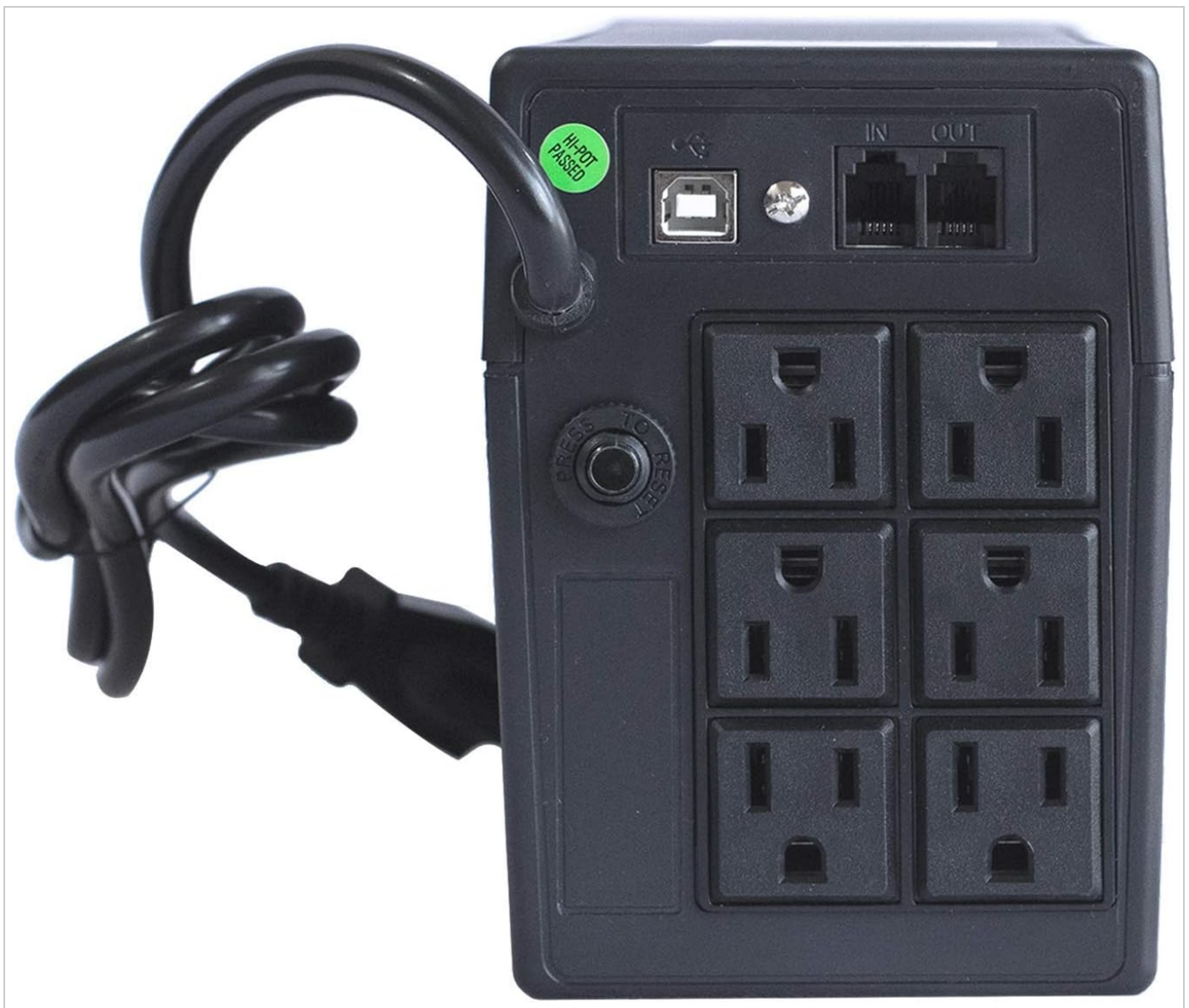
Image 3: Rear view of the Smartbitt SBNB900LCD UPS. This image highlights the back panel of the UPS, showing six NEMA 5-15R outlets, a USB port, and RJ45 input/output ports for telephone line protection. The main power cord is also visible.
