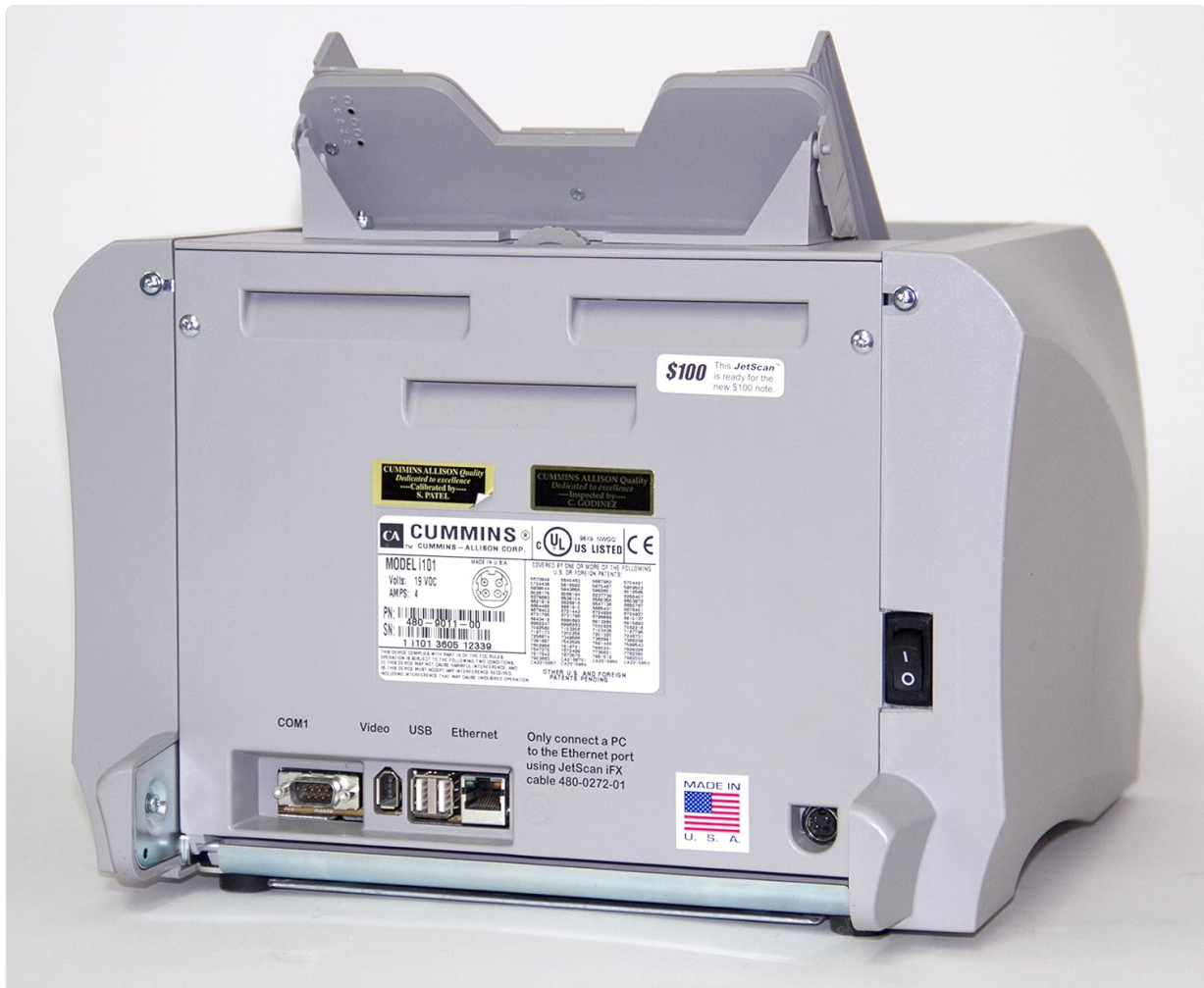
Figure 4.5: Rear View. The rear panel of the JetScan IFX i101, displaying various connectivity options including COM1, Video, USB, and Ethernet ports. The main power switch is located on the right side, and product labels with model and serial information are visible.
