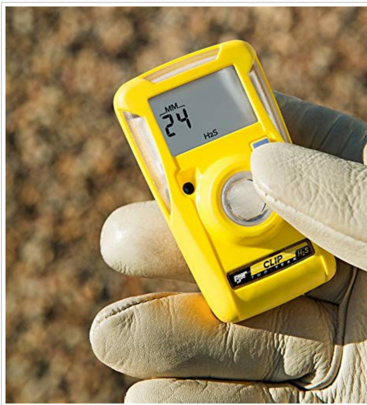
Figure 4: A BW Clip monitor held in a gloved hand, showing a '0' ppm reading for H 2 S (similar display for CO).
