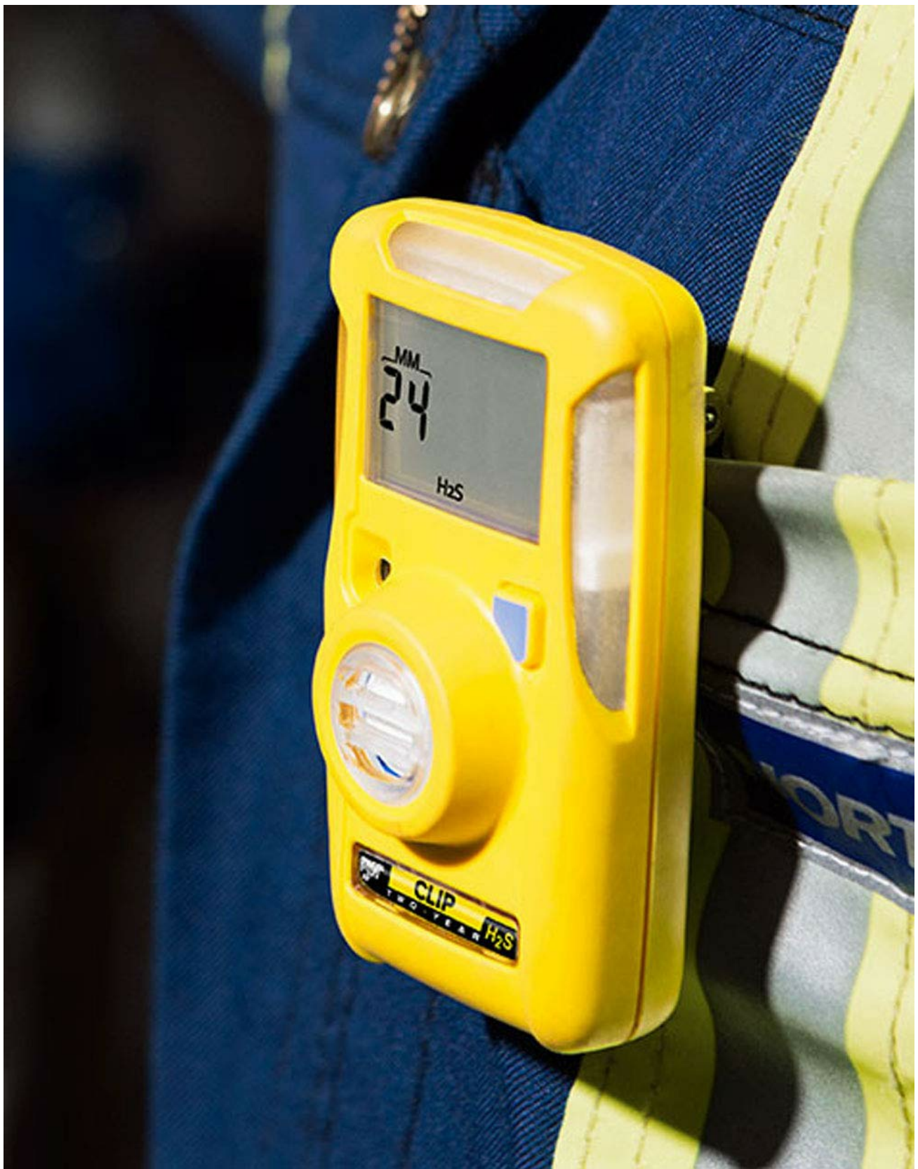
Figure 3: The BW Clip Monitor securely attached to a uniform, demonstrating proper wearing position.
