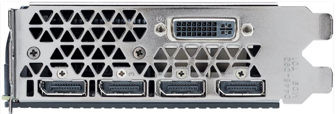
Figure 3.2: The rear I/O panel of the Quadro M6000, featuring four DisplayPort connectors and one DVI port.
