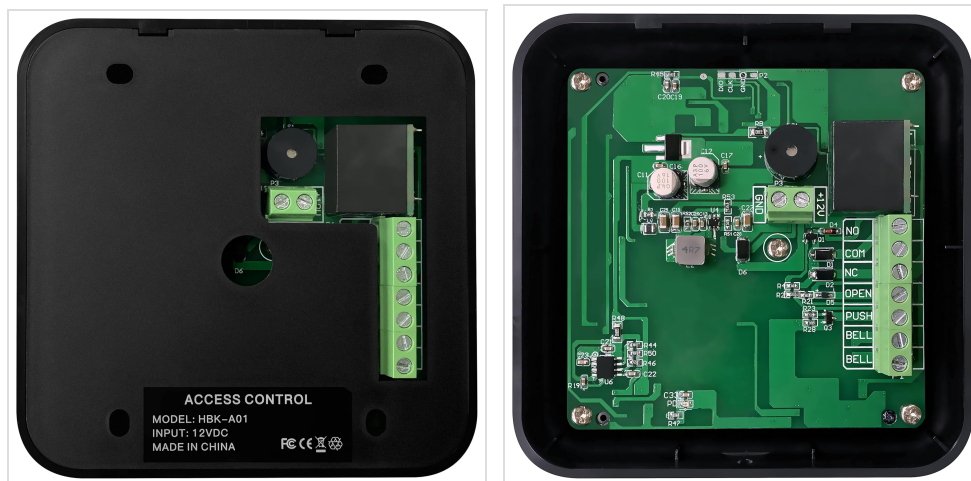
Figure 3: Rear view and internal circuit board of the keypad, highlighting its components.
