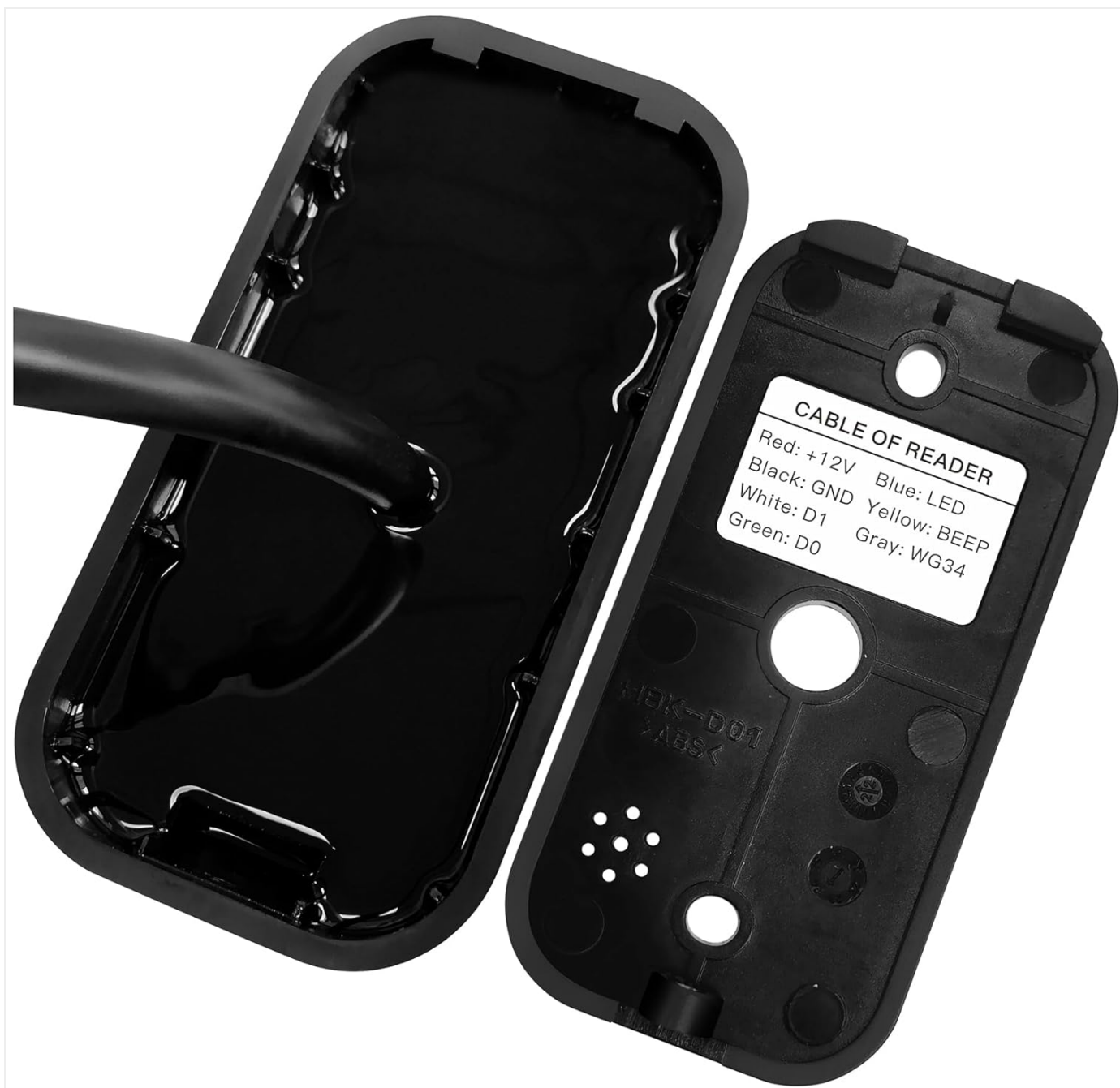
Figure 6.2: Wiring labels on the back cover of the reader. Connections are: Red (+12V), Black (GND), White (D1), Green (D0), Blue (LED), Yellow (BEEP), Gray (WG34).
