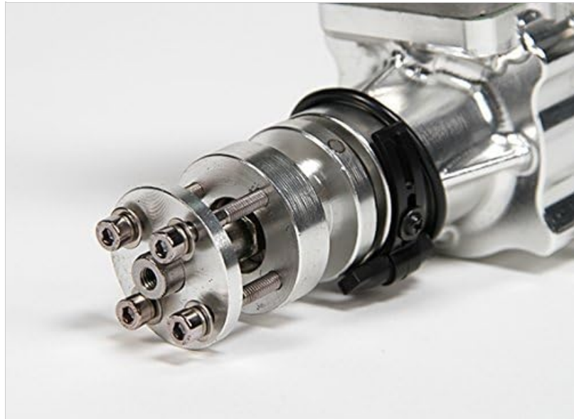
Image 4.2: Close-up view of the propeller mounting hub, showing the bolts for securing the propeller.
