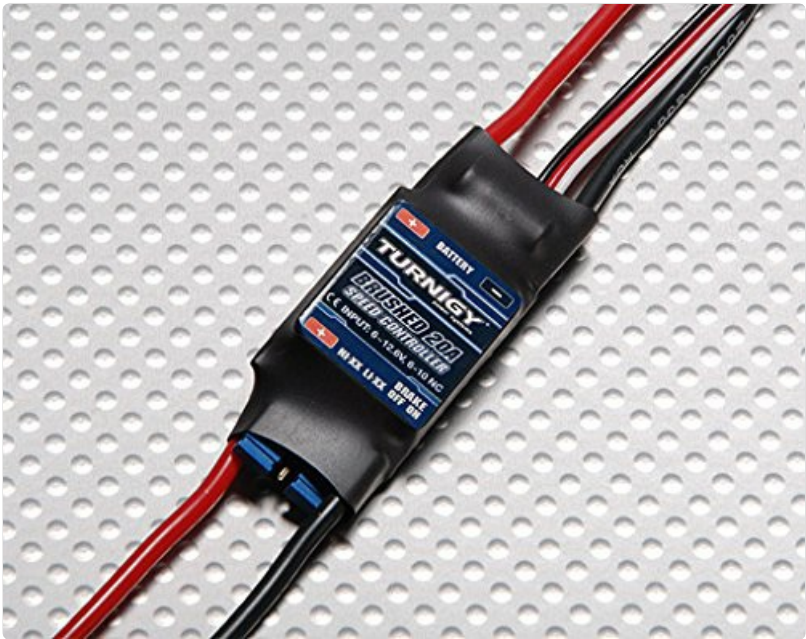
Figure 1: The Turnigy 20A Brushed ESC, showing its compact size and various connection points for motor, battery, and receiver.
