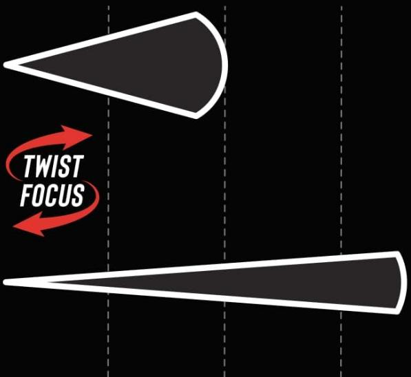
An illustration demonstrating the penlight's focusing beam system, showing the difference between Max View (flood) and Long Distance (spot) beam patterns, adjusted by twisting the head.
