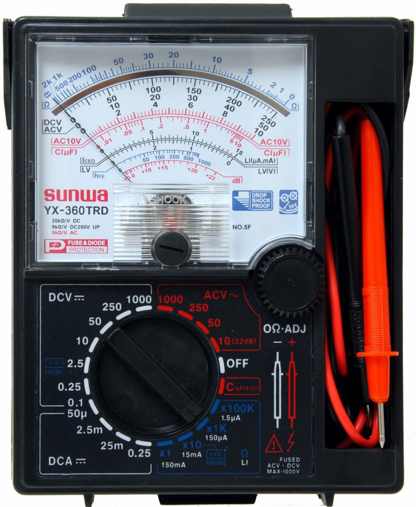
Figure 1: Front View of Multimeter. This image shows the front of the Sunwa YX360-TRD analog multimeter, highlighting its large analog scale, function selector dial, and integrated test leads. The scale displays ranges for DCV, ACV, DCA, Resistance, and Capacitance. The selector dial is prominently positioned for easy function and range selection.
