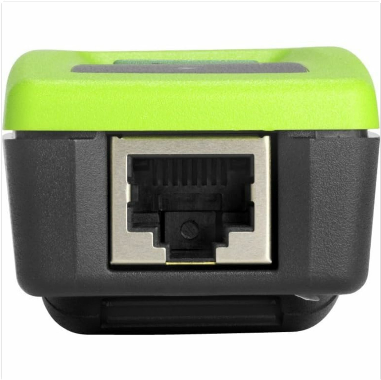
Figure 4: Close-up of the LinkSprinter 300's RJ45 Ethernet port.
