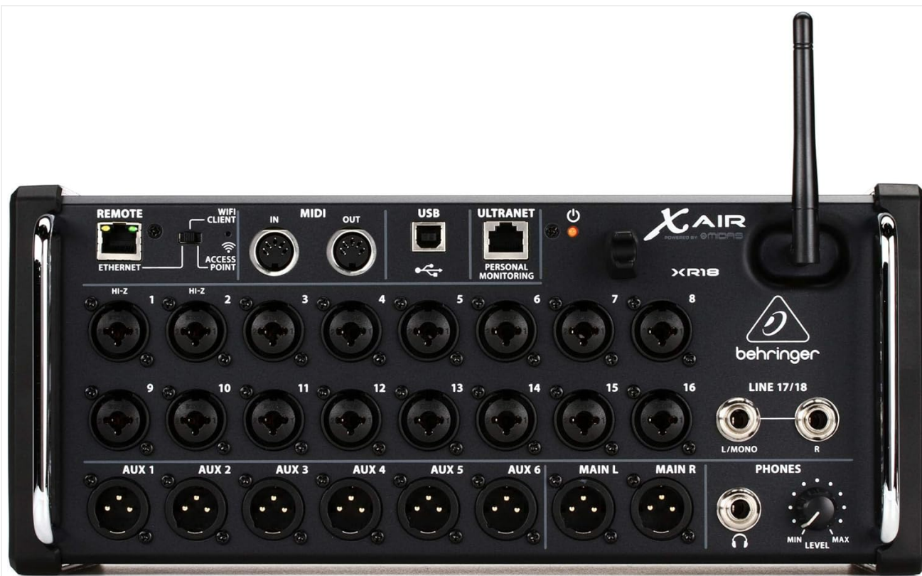
Figure 1.1: Front view of the Behringer X Air XR18, highlighting its comprehensive input and output panel.
