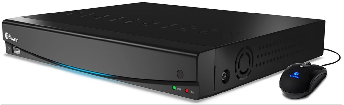
Image 4.1: Front view of the Swann DVR unit with an attached USB mouse for navigation.
