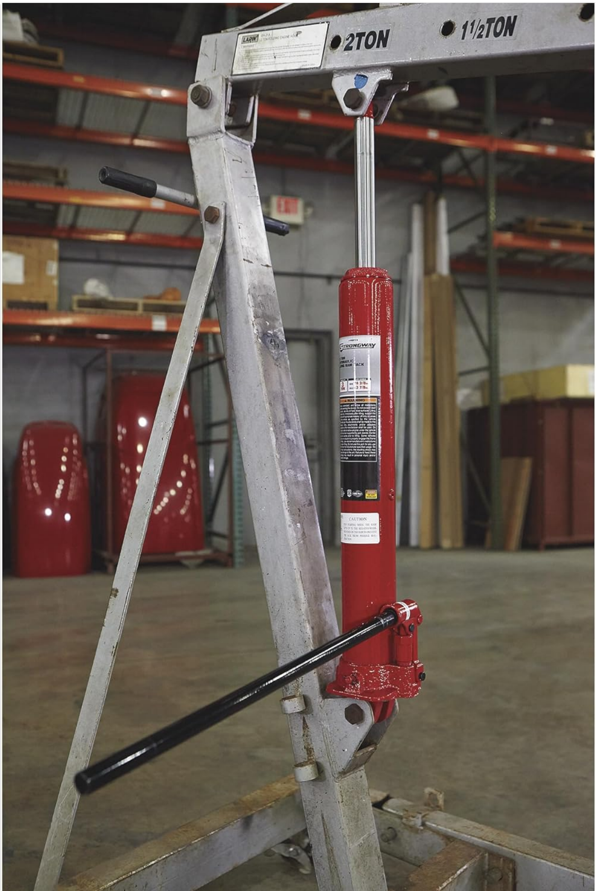
Image: The hydraulic jack integrated into an engine hoist, demonstrating its application for lifting heavy components like an engine.
