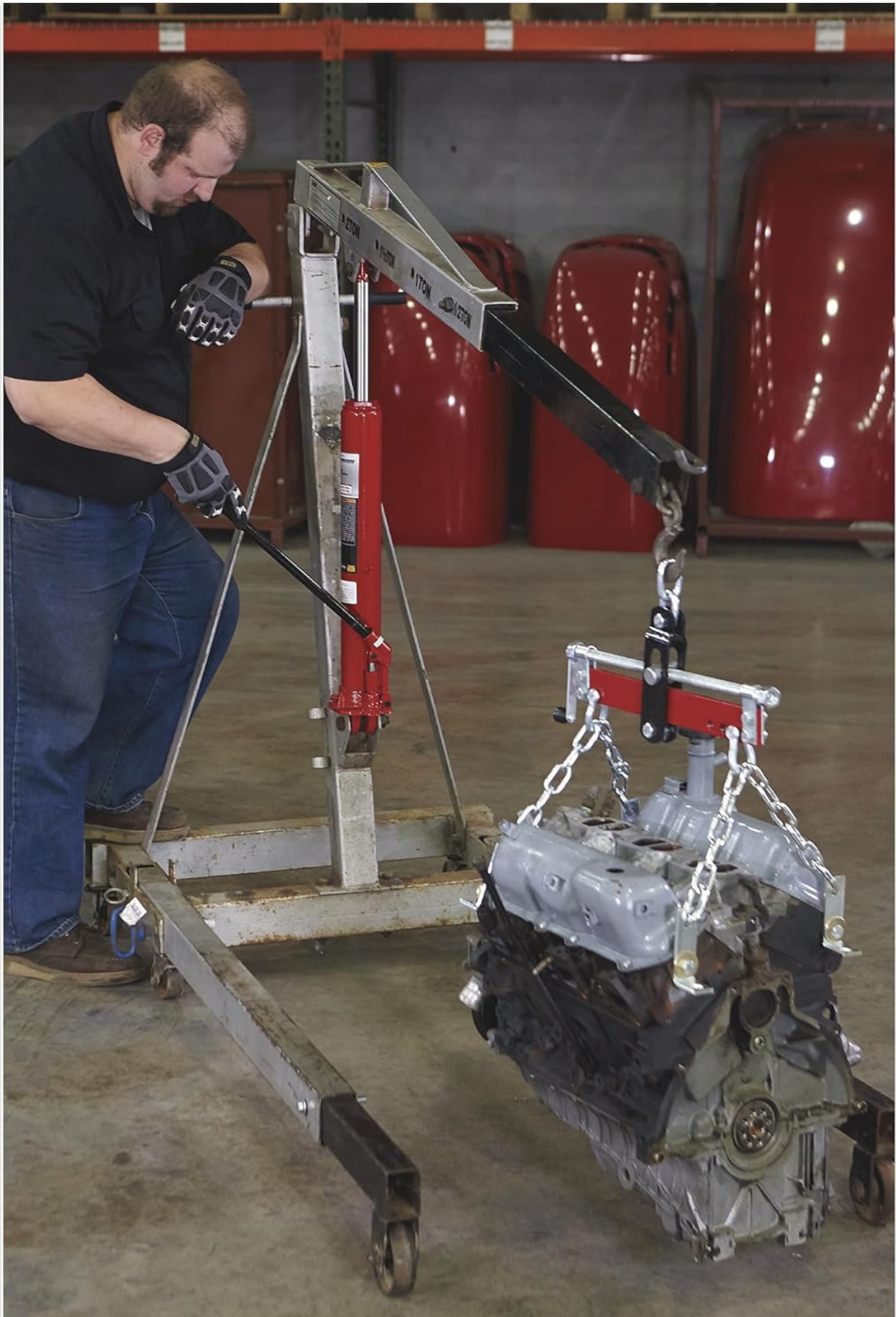
Image: A user operating the hydraulic jack's handle to lift an engine, illustrating the pumping action required for lifting.
