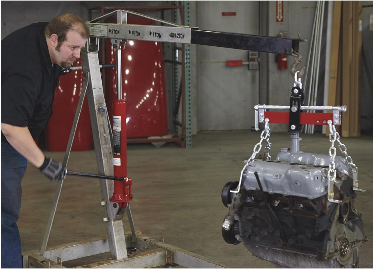
Image: The hydraulic jack actively lifting an engine, demonstrating the jack's extension during the lifting process.
