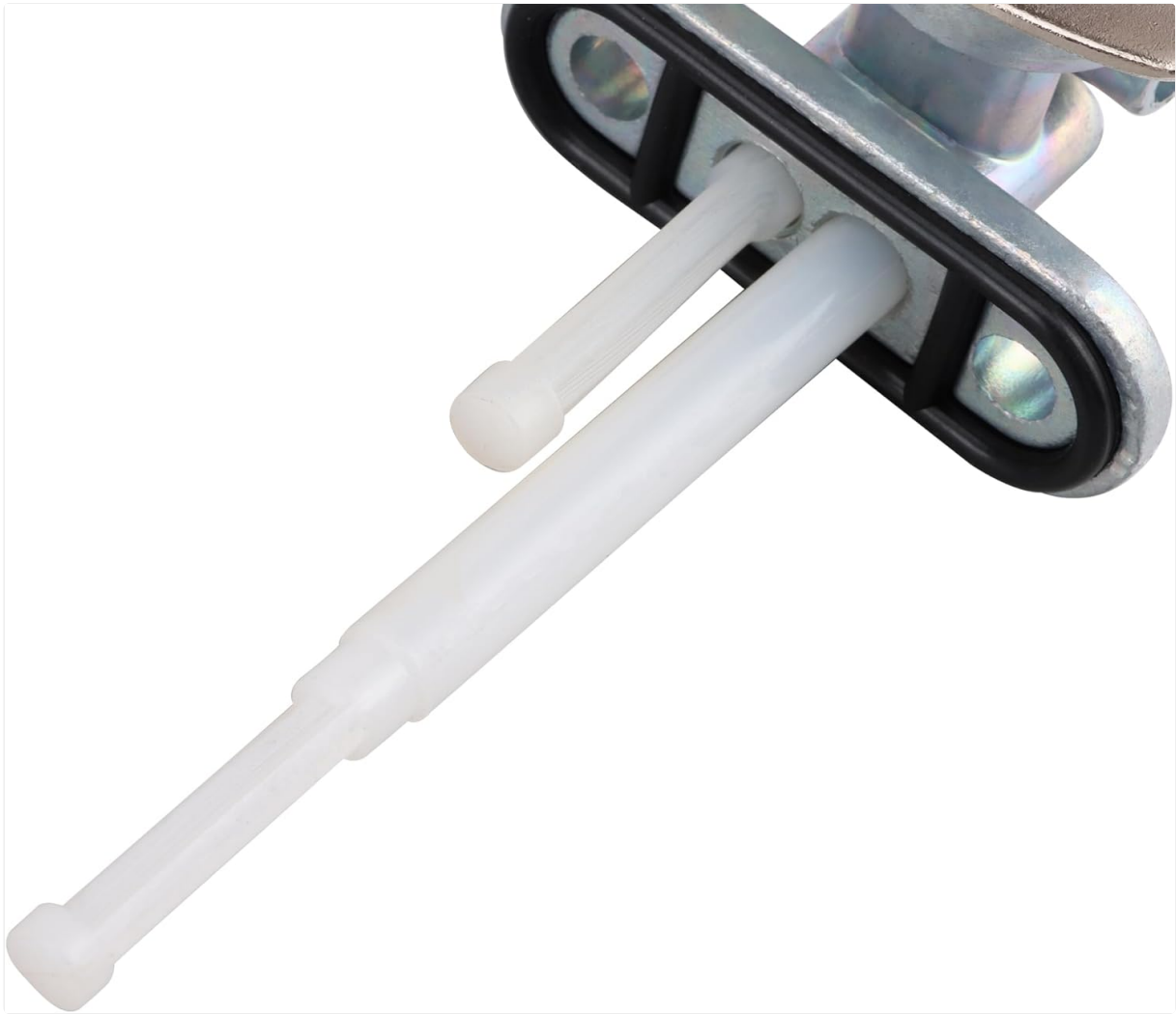
Figure 5: View of the fuel petcock's internal filter screens.
