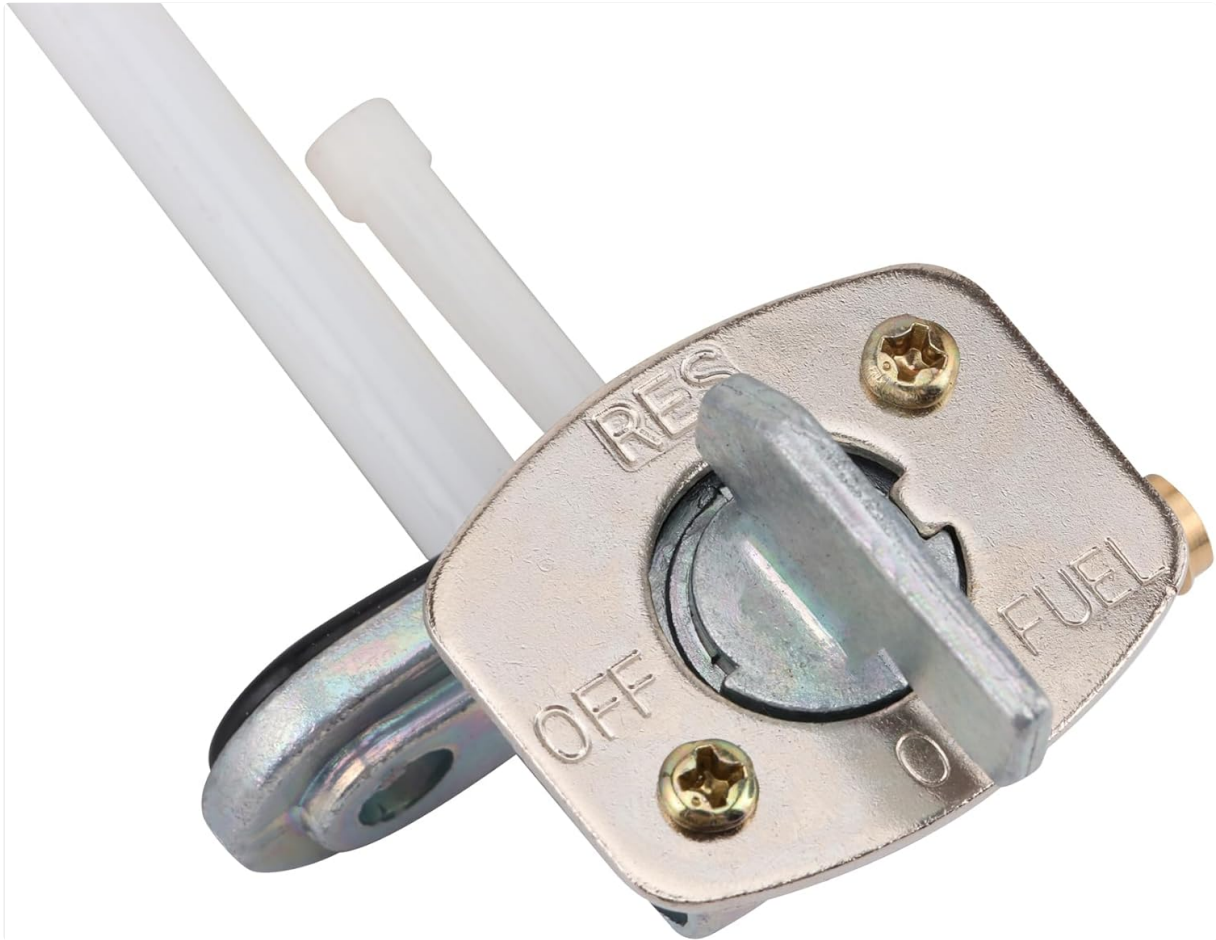
Figure 4: Fuel petcock switch positions (ON, OFF, RESERVE).
