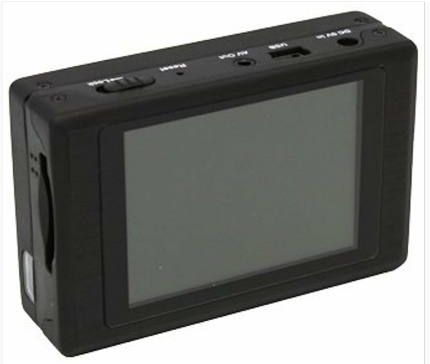
Figure 4.1: DVR Unit Ports and Reset Button
