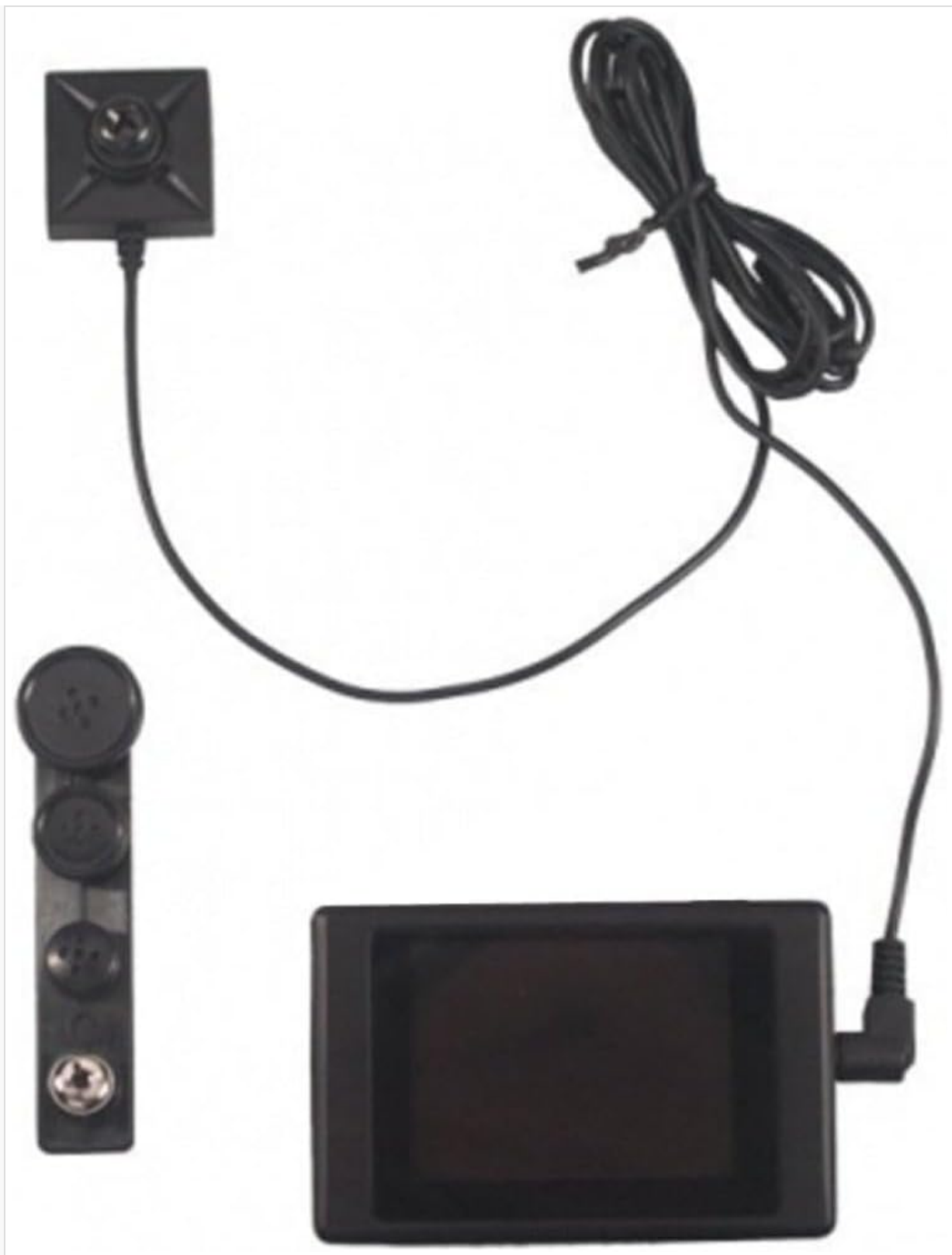
Figure 4.3: DVR Unit with Button Camera Connected
