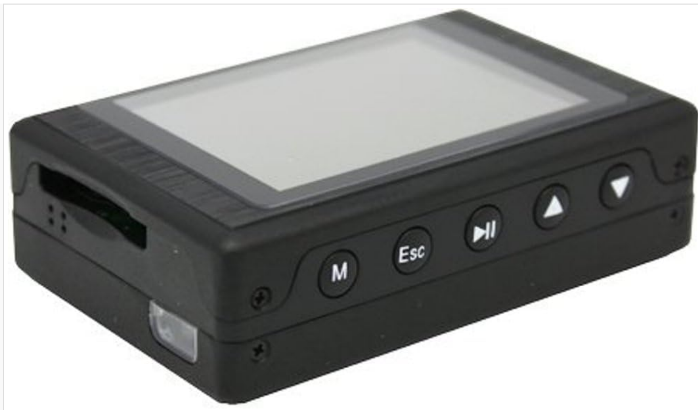
Figure 4.2: DVR Unit Controls and SD Card Slot
