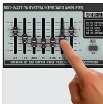
Figure 3.3: Adjusting the 7-band graphic EQ with FBQ feedback detection.
