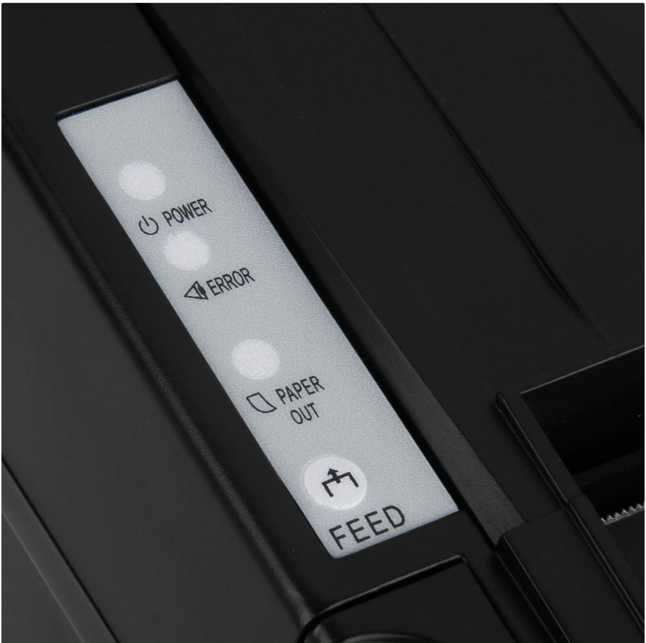
Figure 4.2: Detail of the printer's indicator lights and FEED button.
