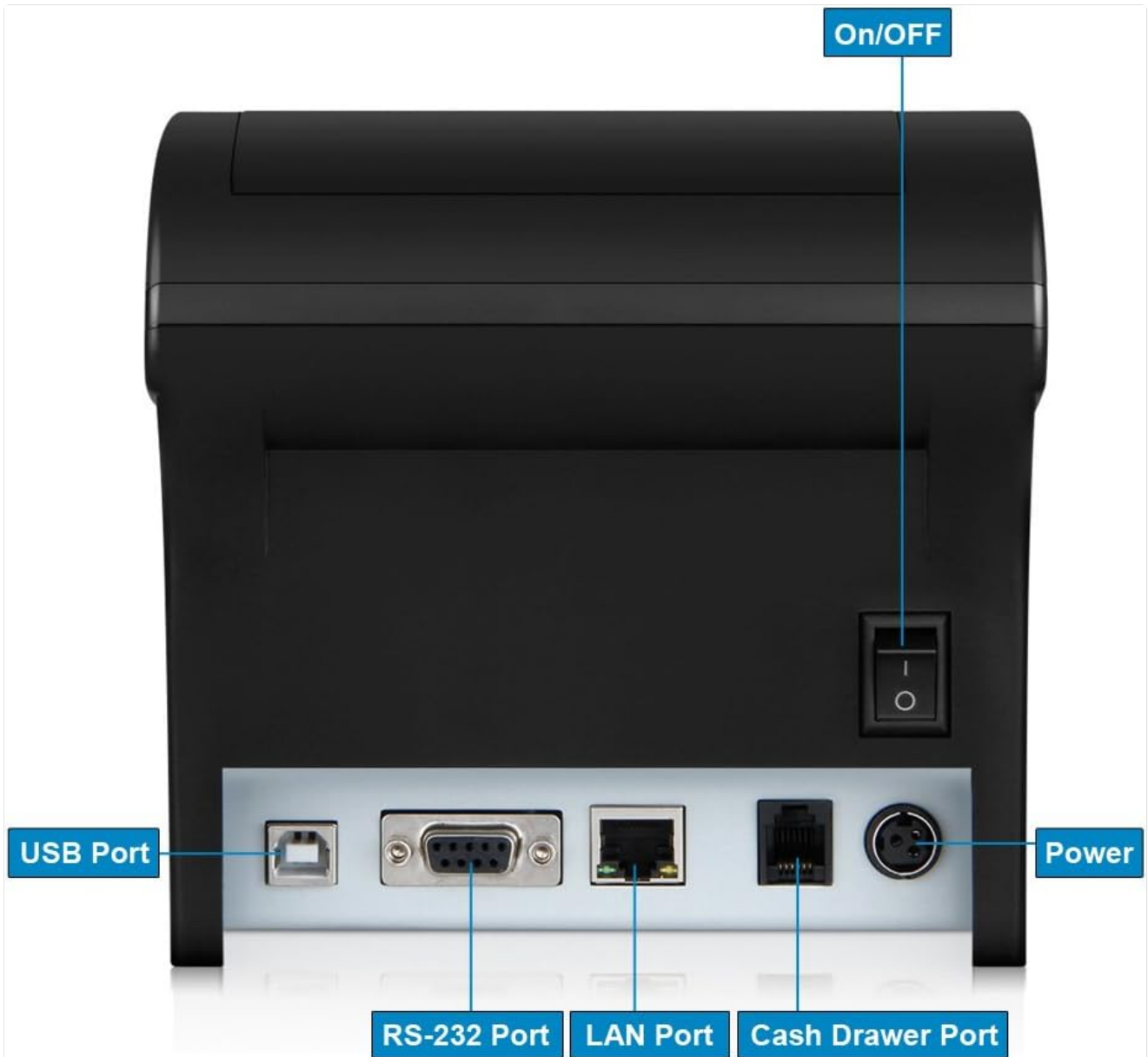
Figure 4.1: Rear panel of the printer detailing all available connection ports and the power switch.
