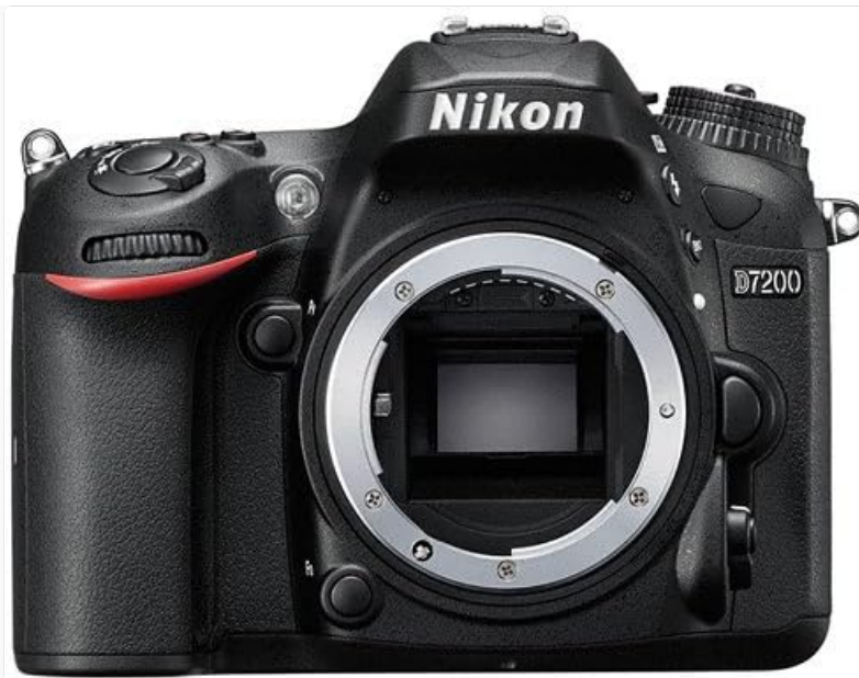
Figure 3.2: Front view of the Nikon D7200 DX-format DSLR Body with the lens removed, exposing the image sensor.
