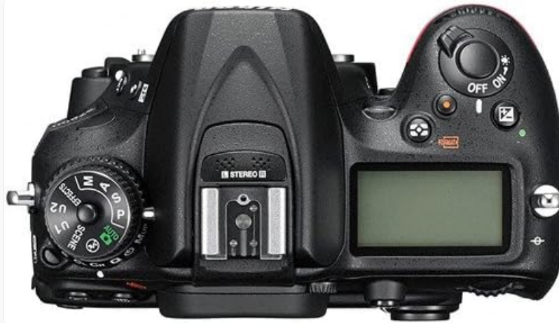
Figure 4.1: Top view of the Nikon D7200 DX-format DSLR Body, showing the mode dial, hot shoe, and top LCD panel.
