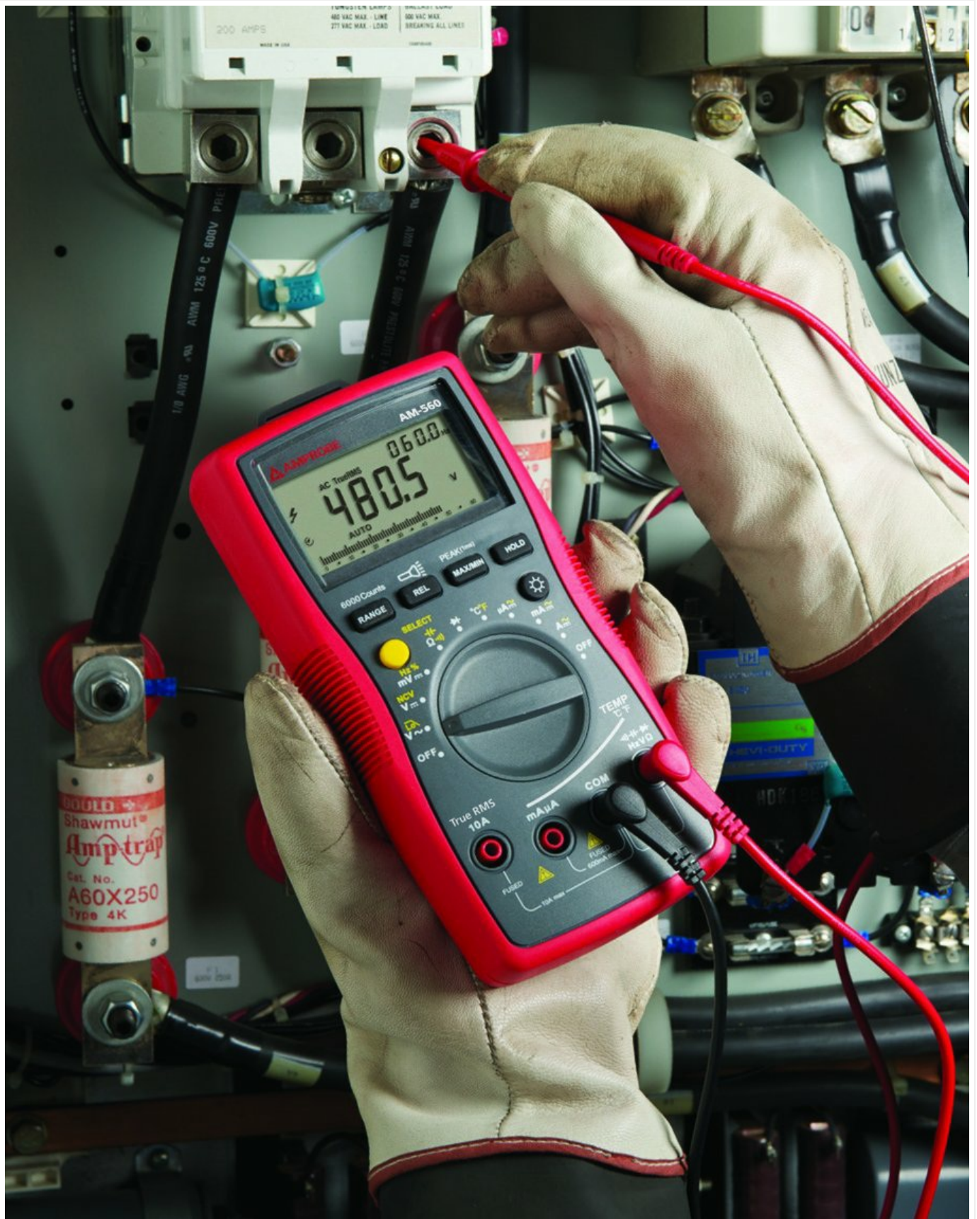
Figure 4.1: Proper connection of test leads to the Amprobe AM-560 multimeter.
