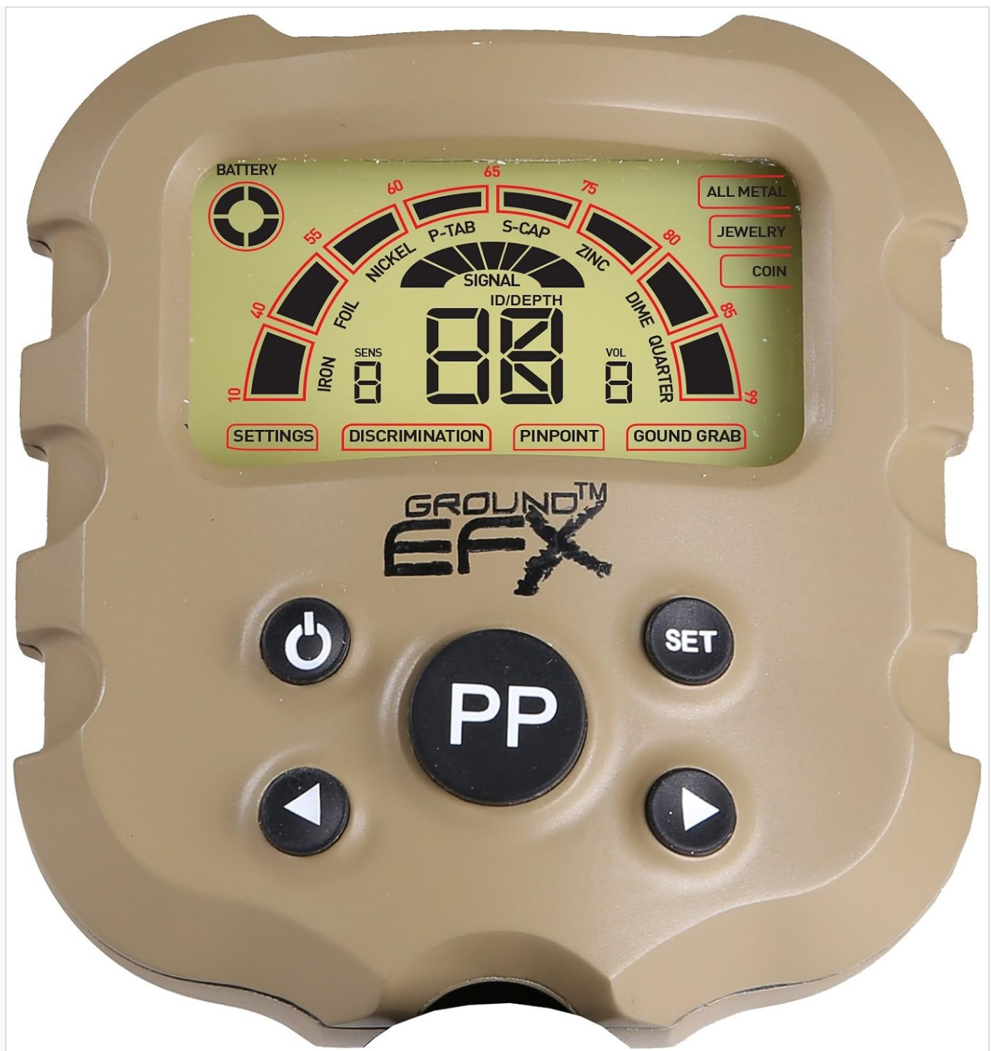
Figure 2: Close-up view of the MX50 control panel. Features include a digital display, power button, pinpoint button (PP), and navigation buttons for settings, discrimination, and ground grab.
