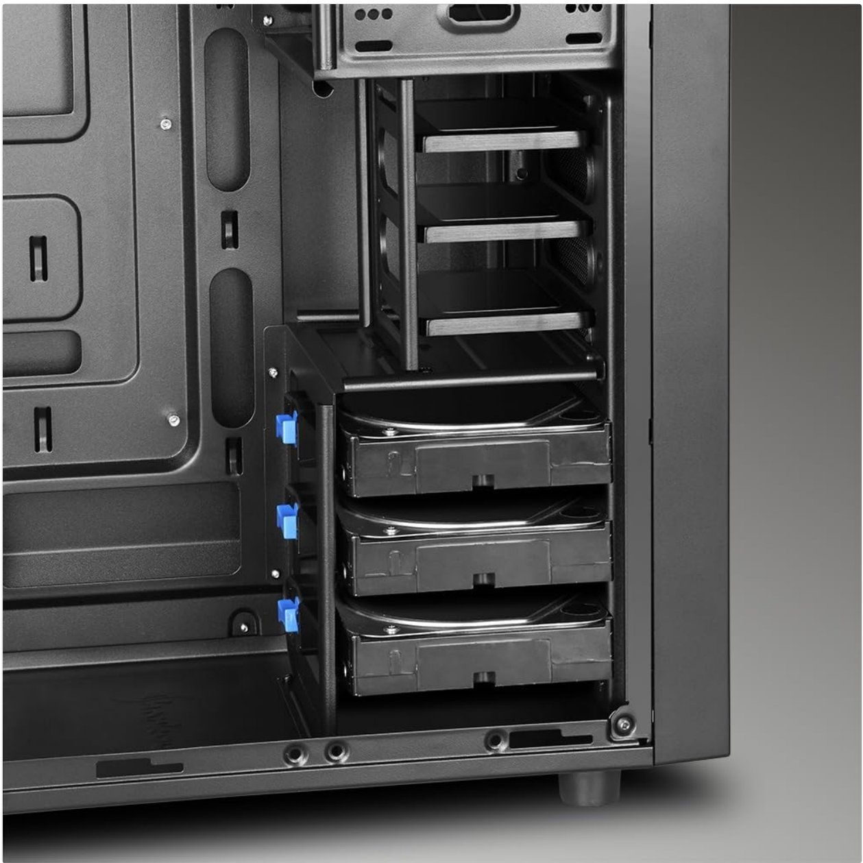
Figure 2.12: Internal drive bays. A view of the internal cages designed to house multiple 3.5-inch hard drives and 2.5-inch solid-state drives, often featuring tool-less installation mechanisms.
