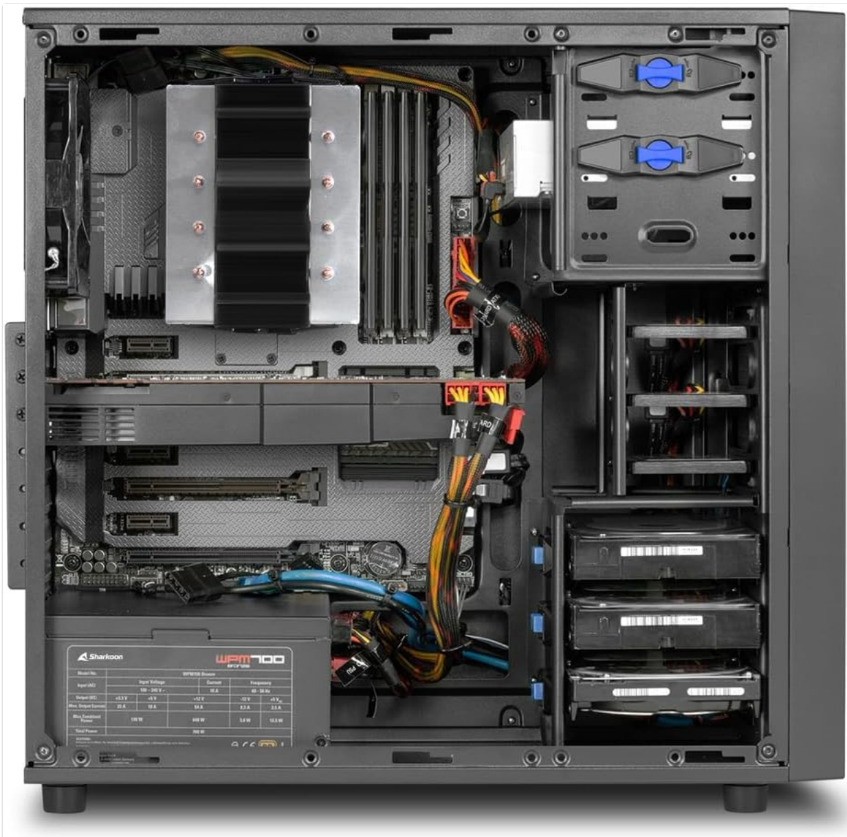
Figure 2.7: Internal layout with components. This image provides a detailed view of the case interior with a motherboard, CPU cooler, graphics card, and drives installed, demonstrating the available space and potential for cable routing.
