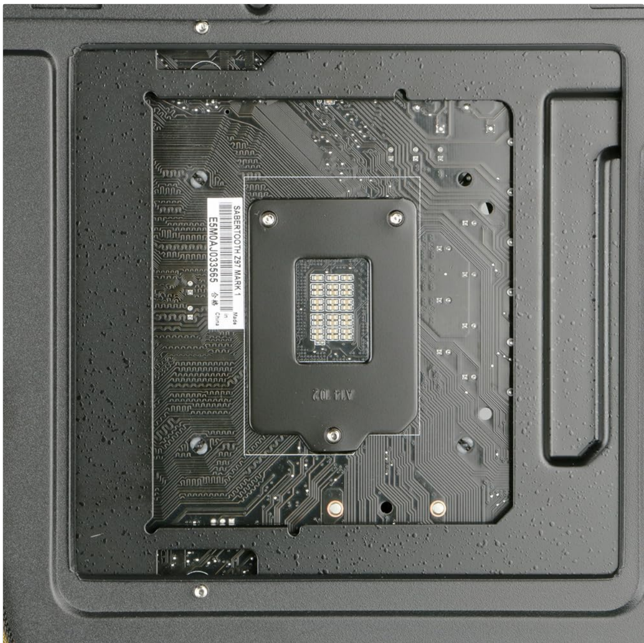
Figure 2.9: CPU cooler installation cutout. This image shows the large cutout on the motherboard tray, allowing for easy installation or removal of CPU coolers without needing to remove the entire motherboard.
