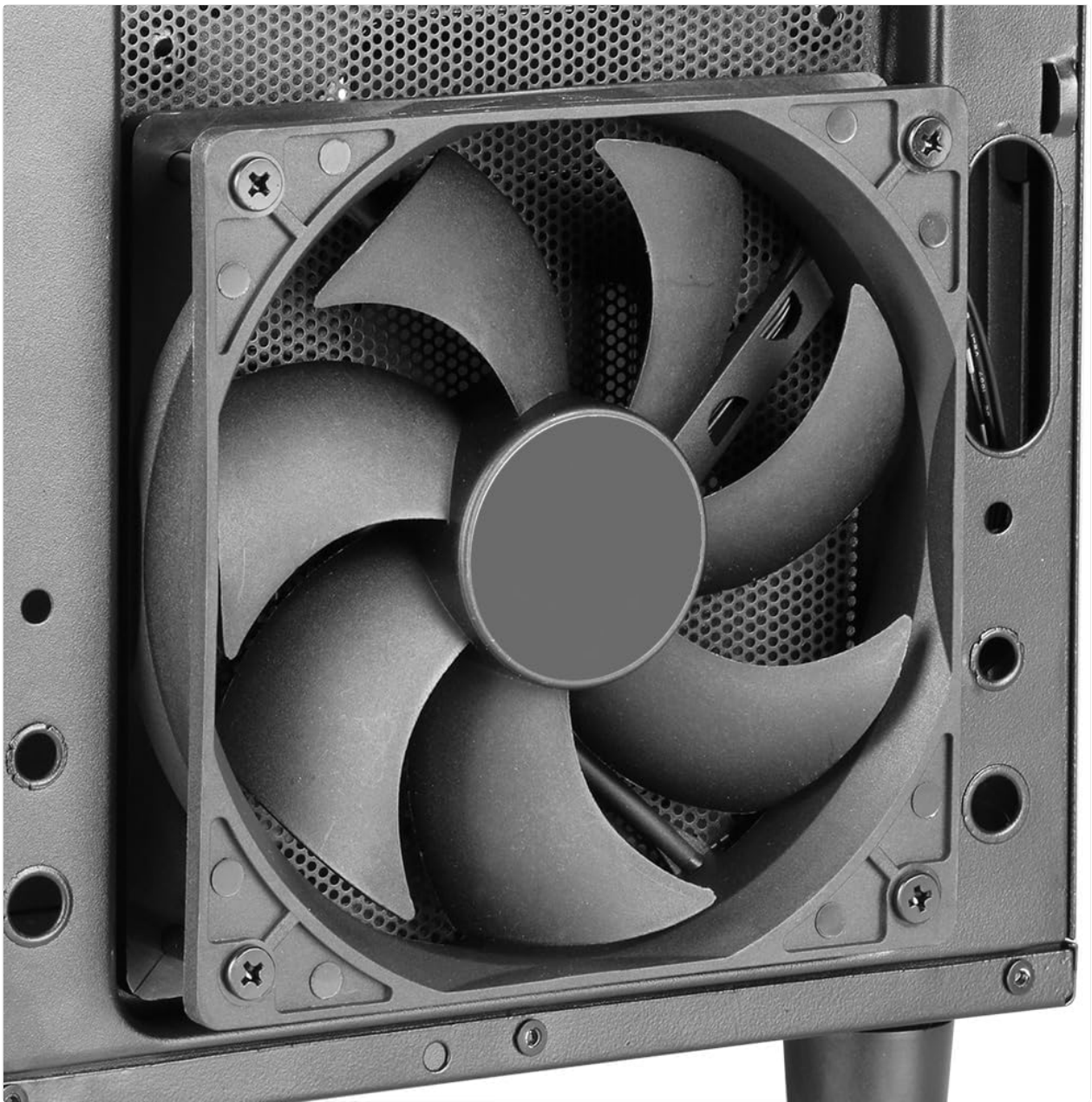
Figure 2.10: Installed 120mm fan. A close-up of a 120mm fan, typically found at the front or rear of the case, responsible for intake or exhaust airflow.
