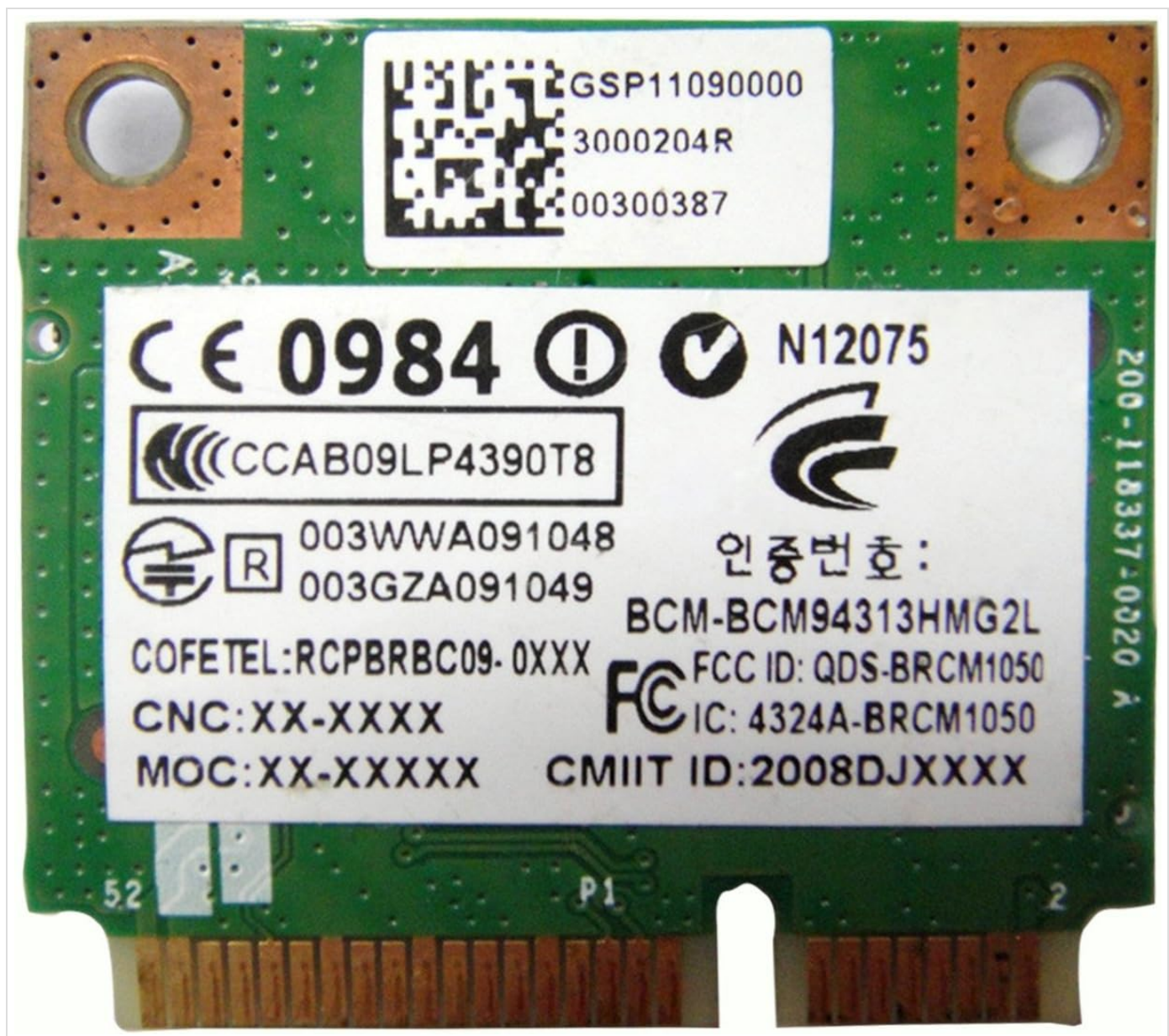
Image 2: Back view of the Broadcom BCM94313HMG2L Half Mini PCI-e WLAN Wireless Card. This side shows various regulatory compliance markings such as CE 0984, N12075, CCAB09LP4390T8, FCC ID: QDS-BRCM1050, and IC: 4324A-BRCM1050. It also reiterates the model BCM-BCM94313HMG2L.
