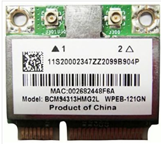
Image 1: Front view of the Broadcom BCM94313HMG2L Half Mini PCI-e WLAN Wireless Card. The label displays the model number BCM94313HMG2L, part number WPEB-121GN, and MAC address 002682448F6A. It also indicates "Product of China". This view shows the main chip and the two antenna connectors at the top.
