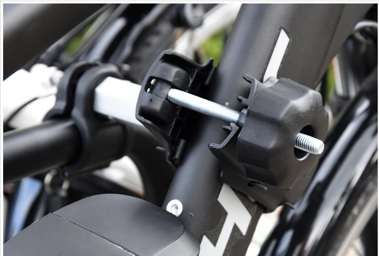
Figure 14: A close-up of the carrier's folding mechanism. This design allows the rack to be collapsed for more convenient storage when not in use.
