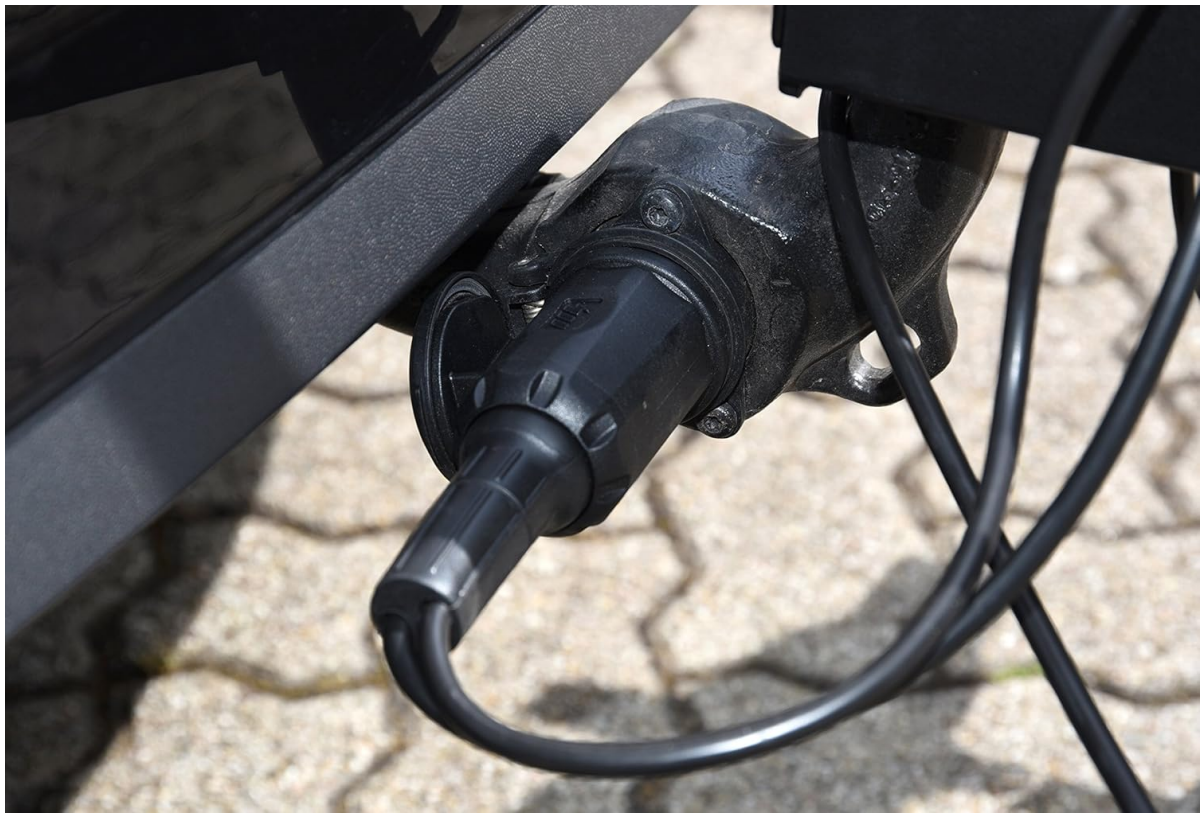
Figure 6: A detailed view of the electrical plug securely inserted into the vehicle's receptacle. A proper connection is vital for the functionality of the carrier's integrated lighting.
