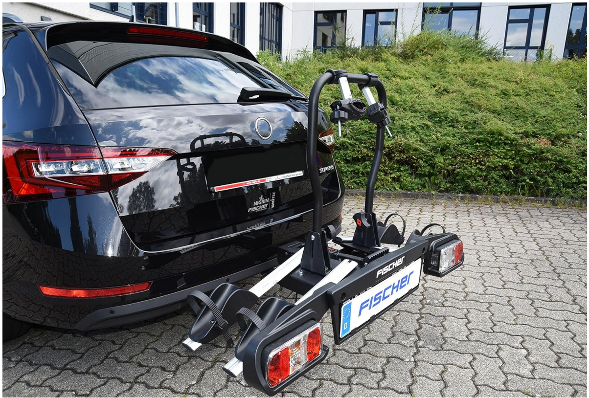
Figure 2: The bicycle carrier rack mounted on the tow bar of a vehicle. This image illustrates the carrier's position when correctly installed on the vehicle.
