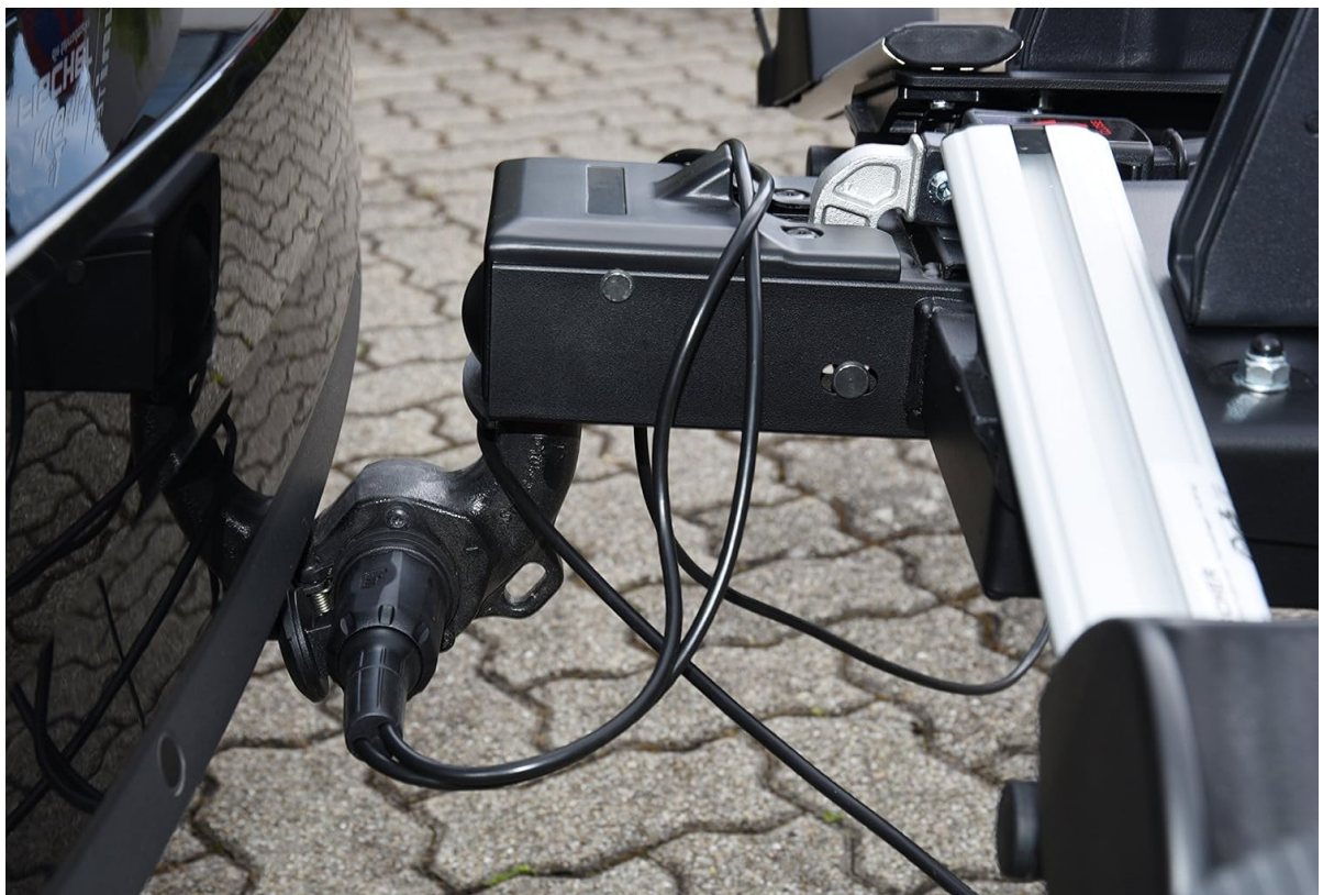
Figure 5: The electrical plug of the carrier connected to the vehicle's tow bar socket. This connection ensures that the carrier's lights function in sync with the vehicle's lighting system.
