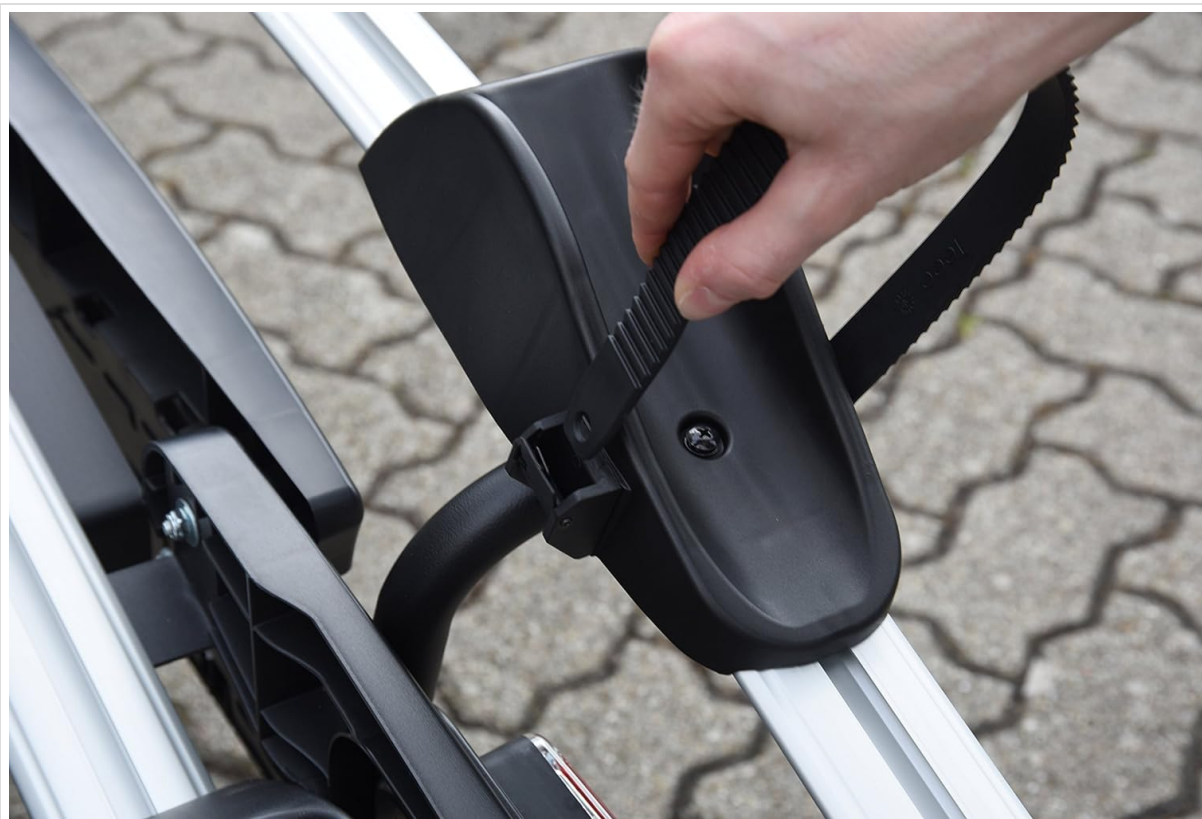
Figure 10: A detailed view of a bicycle wheel secured by an adjustable strap on the carrier's rail. These straps prevent the wheels from moving during transit.
