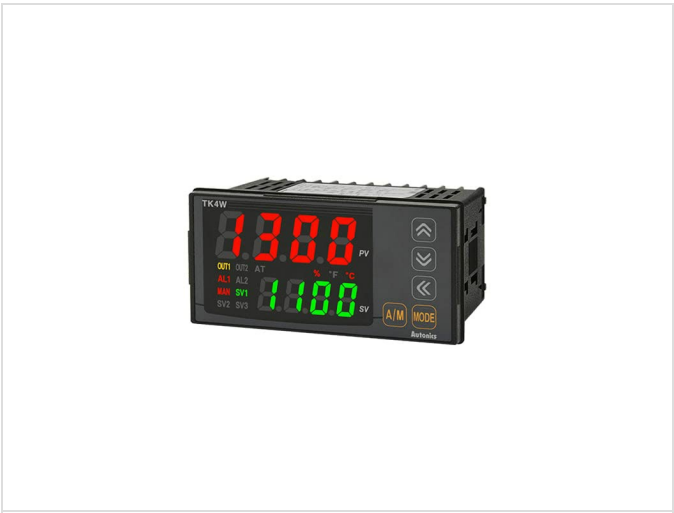
Figure 1: Front panel of the AUTONICS TK4W-14RR Temperature Controller. The image displays the dual digital display, with the upper red display showing the Process Value (PV) and the lower green display showing the Set Value (SV). Indicators for OUT1, OUT2, AL1, AL2, MAN, SV1, SV2, SV3, AT, %°F, and °C are visible. Control buttons for up, down, left/right arrow, and A/M MODE are located on the right side.
