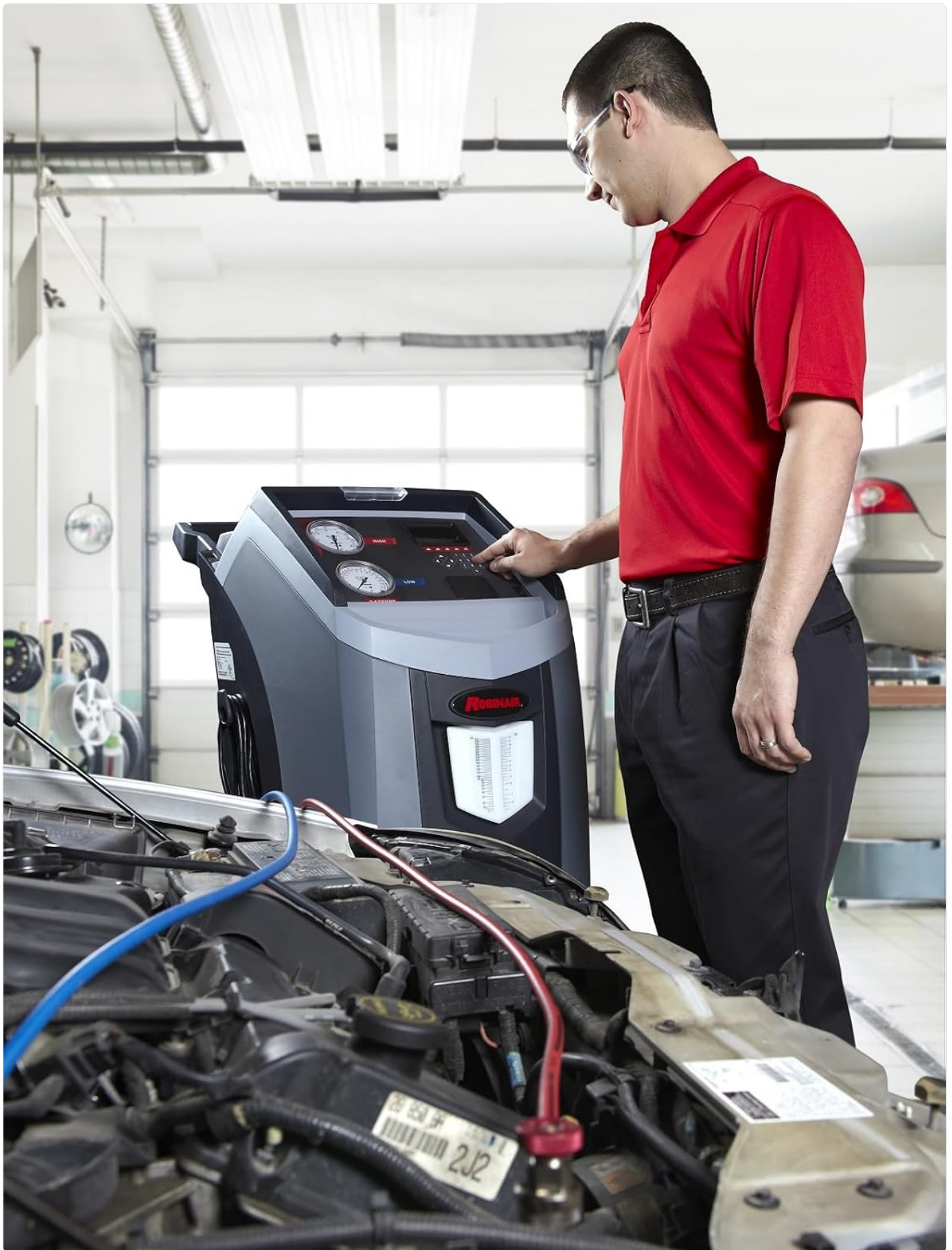
Image: A technician operating the Robinair 34788NI machine, which is connected to an automotive A/C system, demonstrating its use in a workshop environment.
