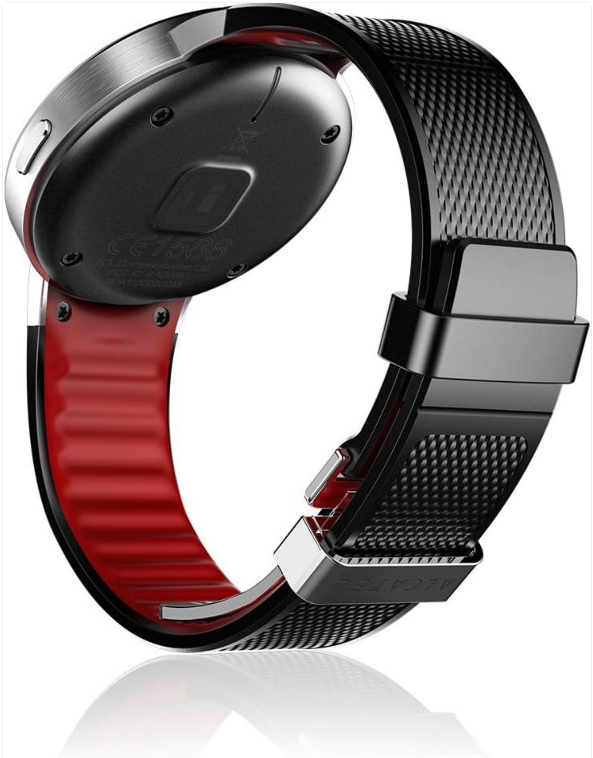
Figure 5: Rear view of the Alcatel One Touch Watch, displaying the heart rate sensor and regulatory markings.
