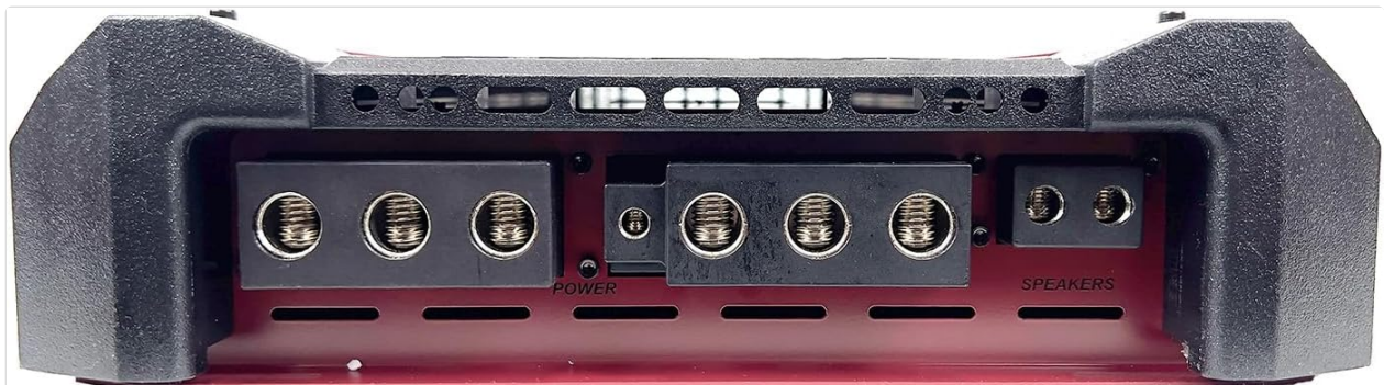
Figure 2: Power and speaker terminal connections on the amplifier.
