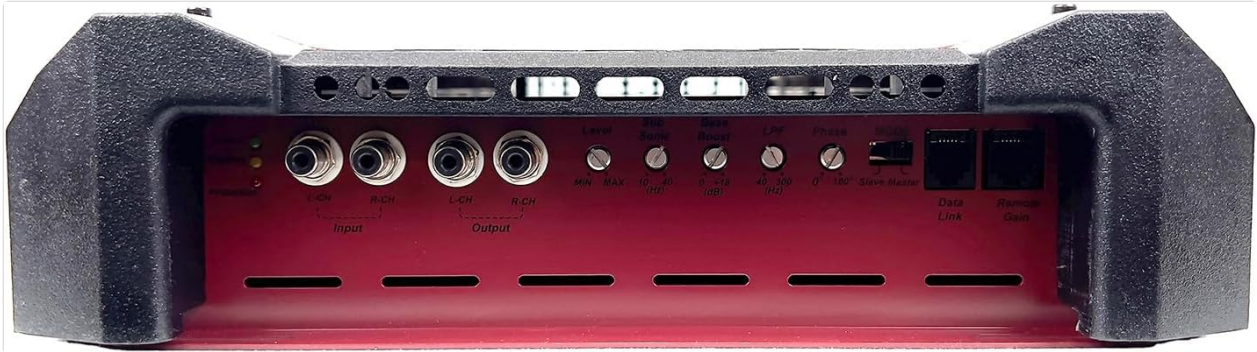
Figure 3: Audio input and control panel of the amplifier.
