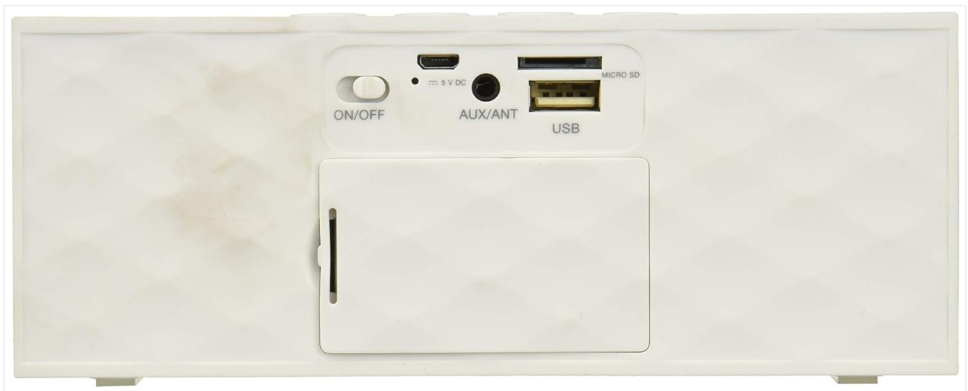
Figure 2.2: Rear Panel of the Fonestar RU-40 Radio. This view highlights the power switch (ON/OFF), 5V DC charging port (Micro USB), AUX/ANT input, USB port, and Micro SD card slot. A battery compartment cover is also visible.
