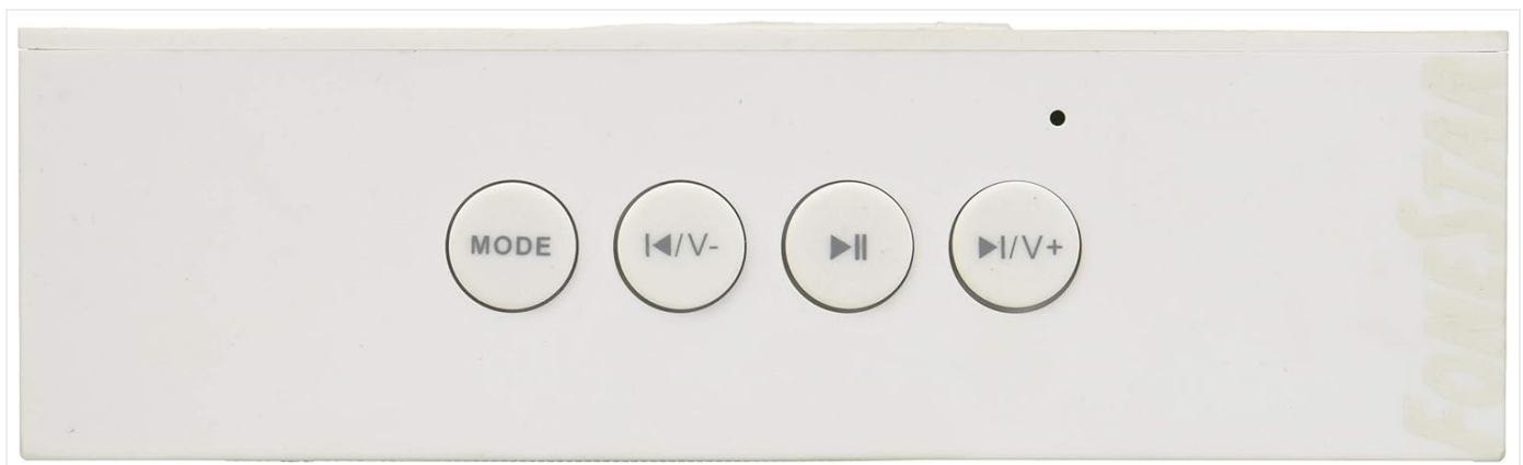
Figure 2.3: Close-up of Top Panel Controls. This image provides a clear view of the four circular buttons: MODE, Previous Track/Volume Down, Play/Pause, and Next Track/Volume Up. An indicator light is also visible.
