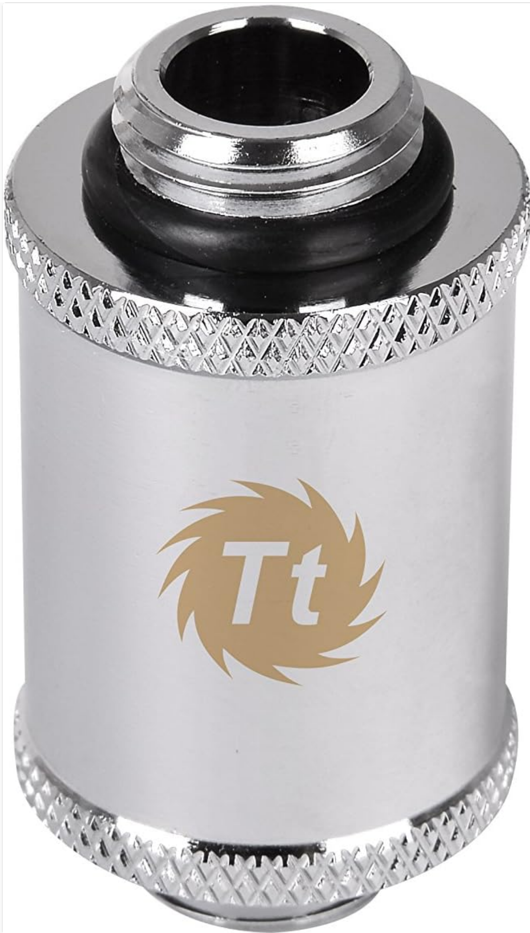
Figure 1.1: Front view of the Thermaltake Pacific G1/4 Male to Male 30mm Extender, showcasing its chrome finish and G1/4 threading with an O-ring.
