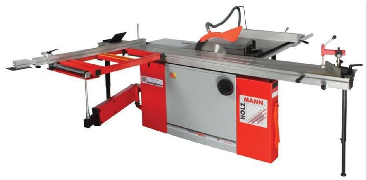
Figure 1: Overview of the Holzmann TS 315VF-2600 Format Saw, showcasing its main components including the sliding table, saw blade, and various fences.
