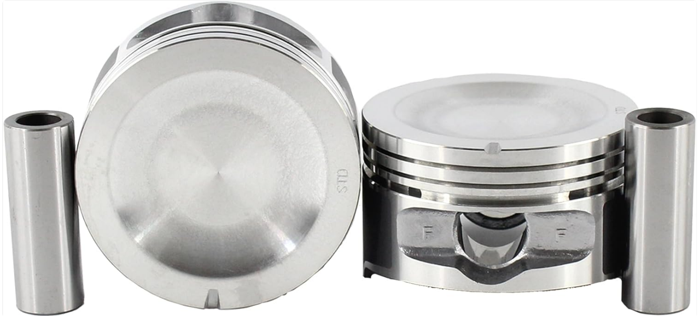
Image: A close-up view of two DNJ P4150 pistons, accompanied by their wrist pins. The image highlights the piston crown, ring lands, and the "STD" marking indicating standard size. This view is useful for verifying part details during installation.
