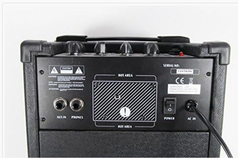
Figure 2: Rear panel connections including AC IN, AUX IN, and PHONES.
