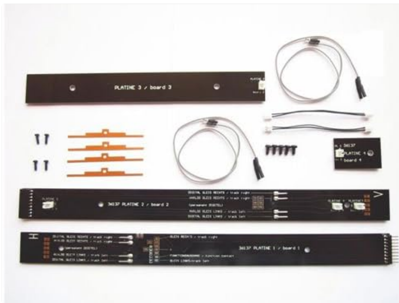
Figure 1: All components included in the Piko 36138 G Scale Interior Light kit. This includes three main circuit boards (labeled "PLATINE 1", "PLATINE 2", "PLATINE 3"), a smaller board ("PLATINE 4"), various connecting wires, four small screws, and four flat, orange conductive strips.
