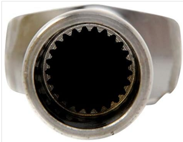
Figure 2: Close-up view of the spline count on the ACP FM-EY001 Drive Shaft Slip Yoke. This image clearly displays the 25 internal splines, which are essential for proper engagement with the transmission output shaft.
