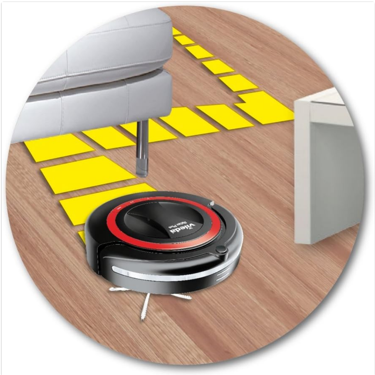
Image 5.1: The Vileda Relax Plus demonstrating its obstacle detection capabilities, indicated by yellow wave patterns, as it approaches furniture.
