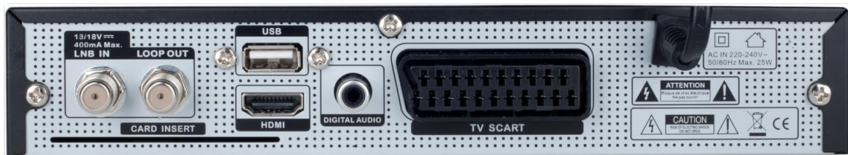
Image 2: Rear panel of the Telestar TD 2300 HD+ receiver, showing various input and output ports.
